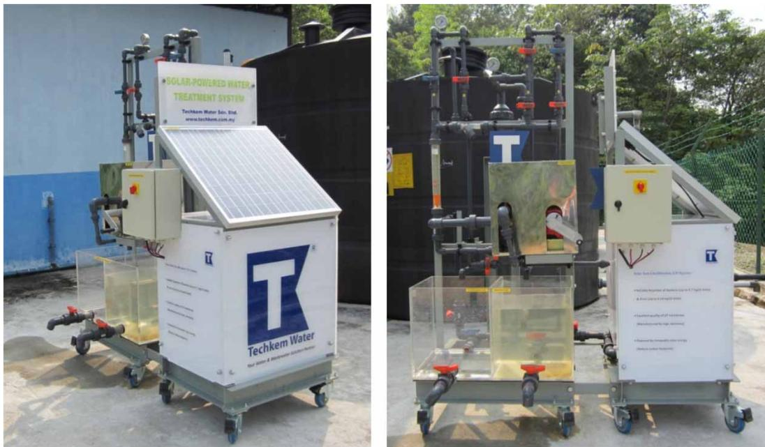
Figure 1 | Solar-powered ultrafiltration membrane water treatment system.
