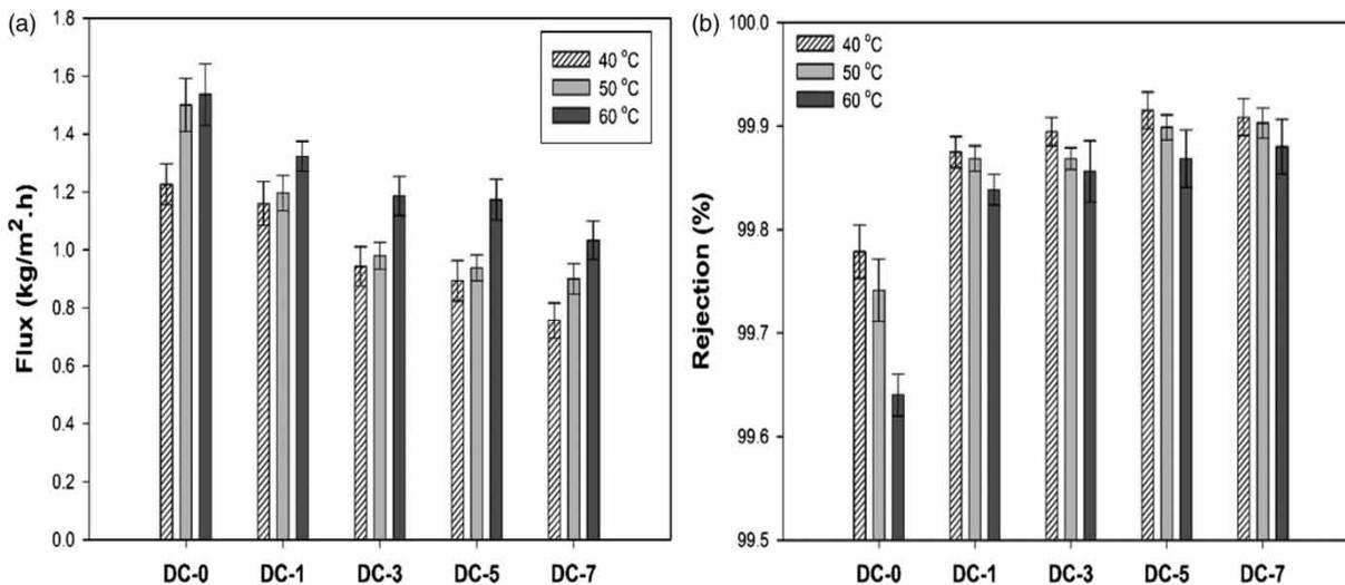
**Figure 2** | Effect of dip-coating numbers on water flux and total salt rejection factor at constant temperature.
