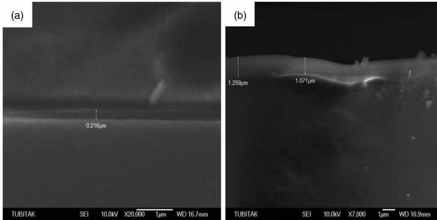
**Figure 1** | SEM micrographs of (a) one-time and (b) seven-times PEBA-coated PVA membranes.
