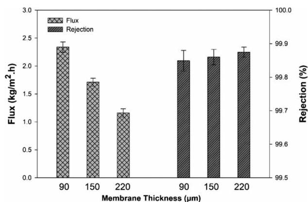
Figure 3 | Effect of membrane thickness on flux and rejection.
