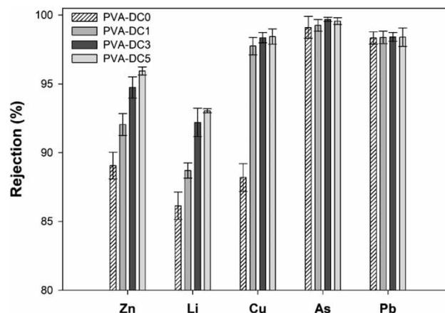
Figure 4 | Rejection of heavy metals.
