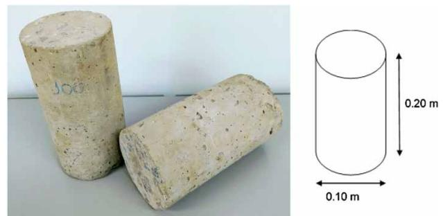
Figure 1 | Concrete samples.
