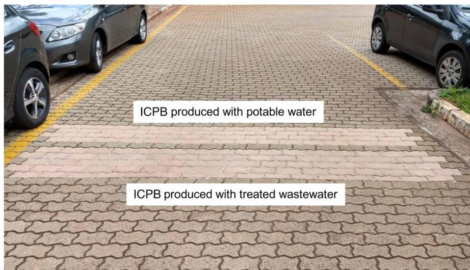
**Figure 2** | Interlocking concrete paver blocks (ICPB) produced with treated wastewater and potable water being tested in the parking lot.
