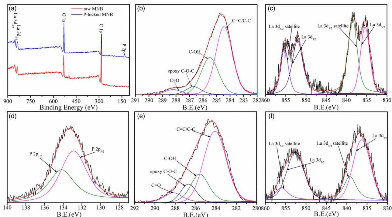
**Figure 2** | XPS analysis of the pristine and used MNB: (a) XPS survey, (b) C 1s of MNB, (c) La 3d of MNB, (d) P 2p of the used MNB, (e) C 1s of the used MNB, and (f) La 3d of the used MNB.
