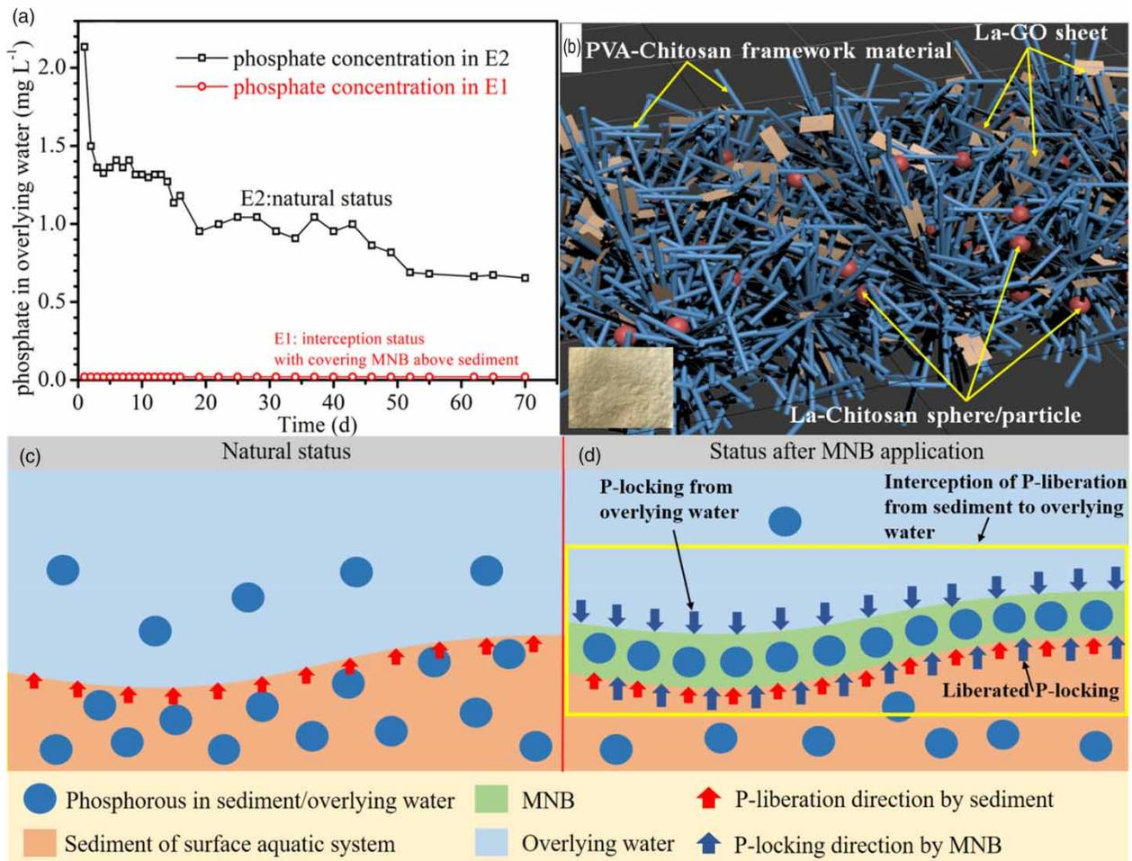
**Figure 5** | (a) The performance of phosphate interception by covering MNB; (b) schematic diagram of MNB structure; (b-inset) photograph of the pristine MNB; (c) the natural status of phosphate liberation in a surface aquatic system; and (d) interception status of phosphate liberation by MNB.
