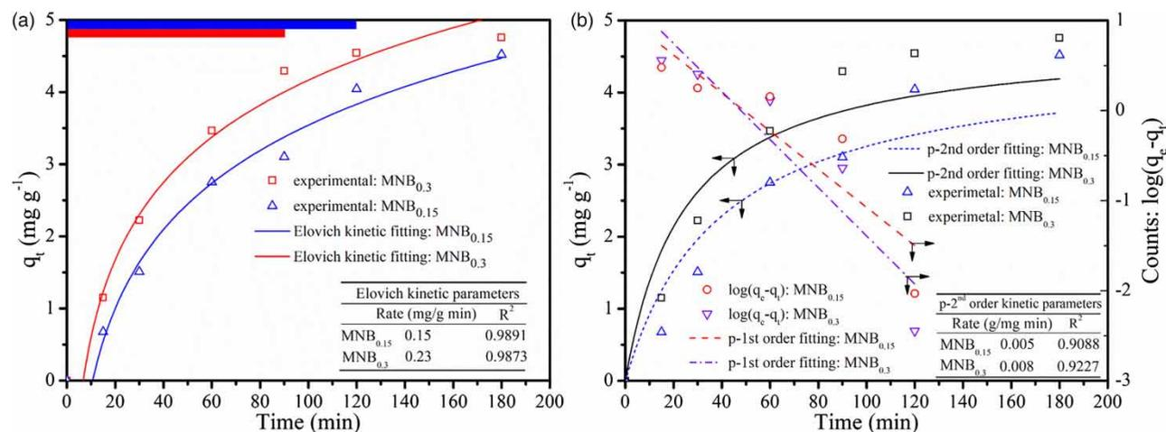
**Figure 3** | Kinetics and effect of contact time of phosphate binding by MNB, (a) Elovich fitting and (b) pseudo-1st/2nd order fitting. Please refer to the online version of this paper to see this figure in colour: <http://dx.doi.org/10.2166/ws.2019.151>.
