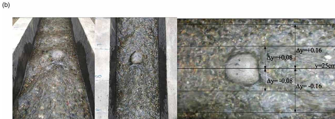
Figure 2 | General arrangements of the boulder bed flow structure experiment: (a) hydrodynamics investigation; (b) bed morphology characteristics investigation.
