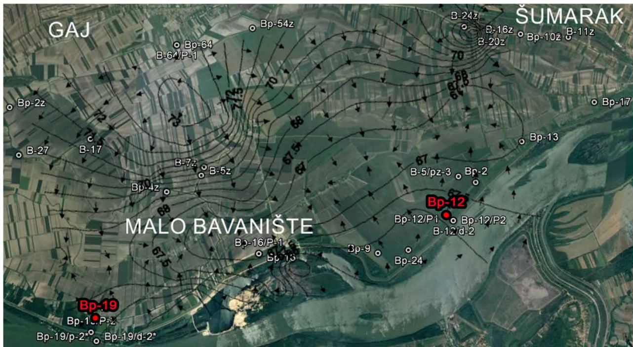
Figure 3 | Kovin-Dubovac drainage system groundwater table levels, expressed in metres above sea level, with highlighted wells selected for pesticide concentration monitoring (Bp-12 and Bp-19); arrows indicate groundwater movement.
