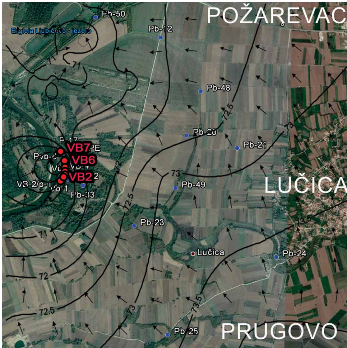
Figure 4 | Groundwater table levels at the Ključ groundwater source, expressed in metres above sea level; dots placed close to each other represent pumping wells with specifically highlighted wells selected for pesticide concentration monitoring (VB2, VB6 and VB7); dots with labels starting with 'Pb' represent observed piezometers; arrows indicate groundwater movement.
