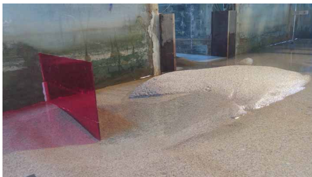
Figure 6 | Experimental view of flow and bed deformation in Test 2.
