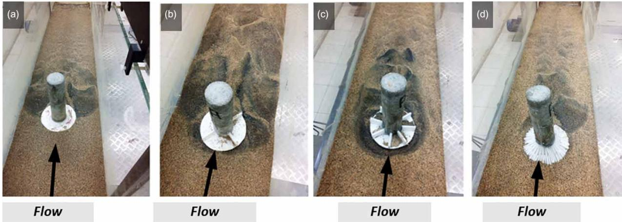
**Figure 8** | Photographs of equilibrium scour depths resulting from flow around bridge piers with different types of collars: (a) flat collar; (b) wing collar 90°; (c) wing collar 45°; and (d) conical collar.
