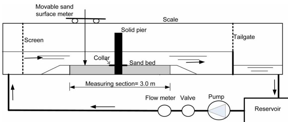
Figure 2 | Experimental flume set-up.
