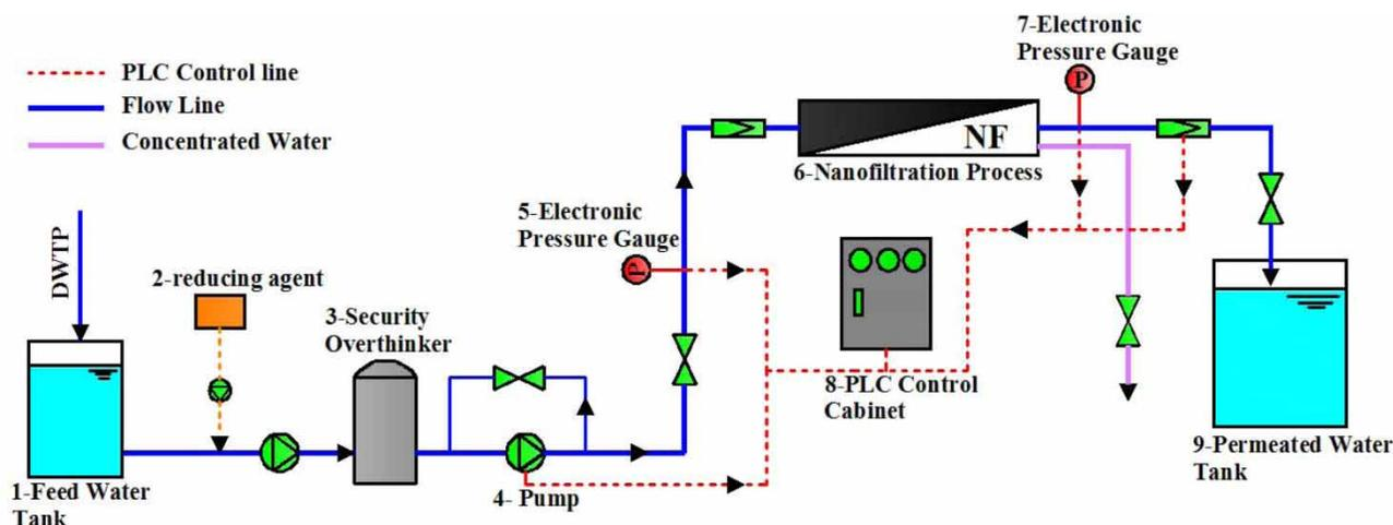
Figure 1 | A schematic diagram of the pilot-plant system.
