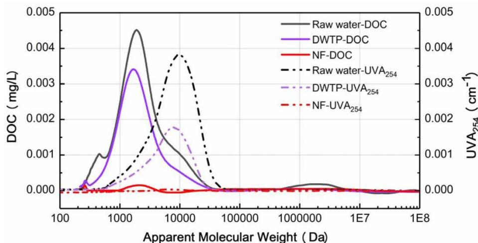
**Figure 4** | Representative HPSEC chromatograms highlighting the MW distribution of DOC and UVA<sub>254</sub> for each sample.
