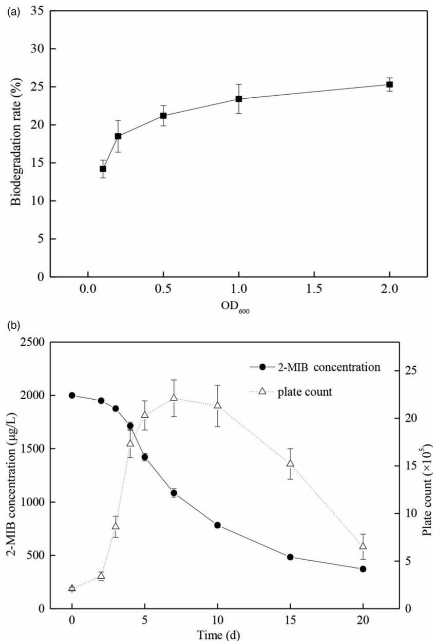
**Figure 3** | Effect of degrader dosage on the degradation of 2-MIB: (a) effect of degrader dosage on 2-MIB (20  $\mu\text{g/L}$ ) degradation in the third day; (b) growth curve of degraders during 2-MIB (2 mg/L in MSM) degradation.
