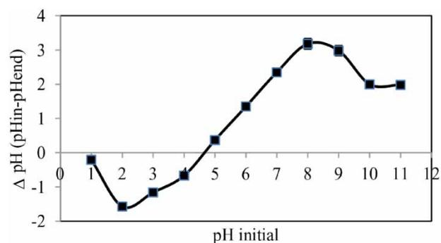
**Figure 4** | Zero-point charge of AL-ZMR beads.
