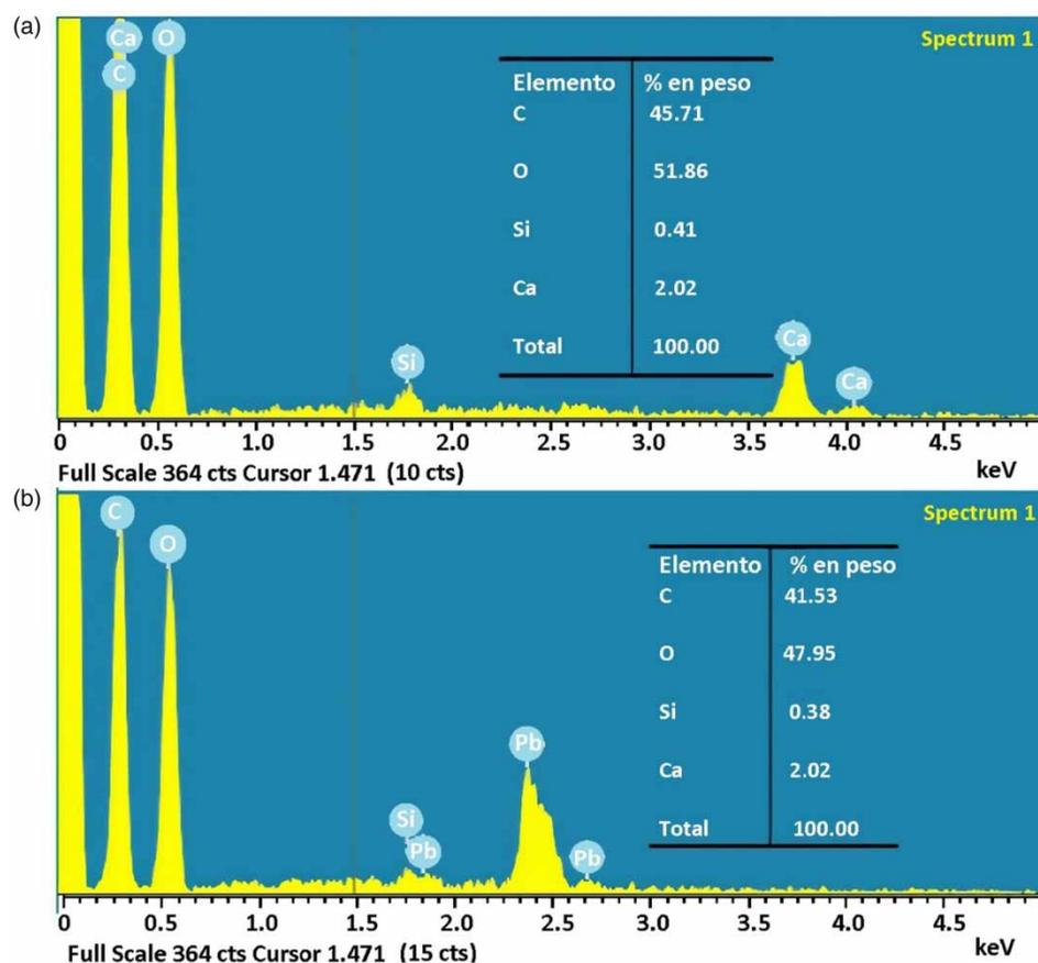
**Figure 2** | EDS analysis of AL-ZMR: (a) before and (b) after the adsorption of Pb (II) ions.
