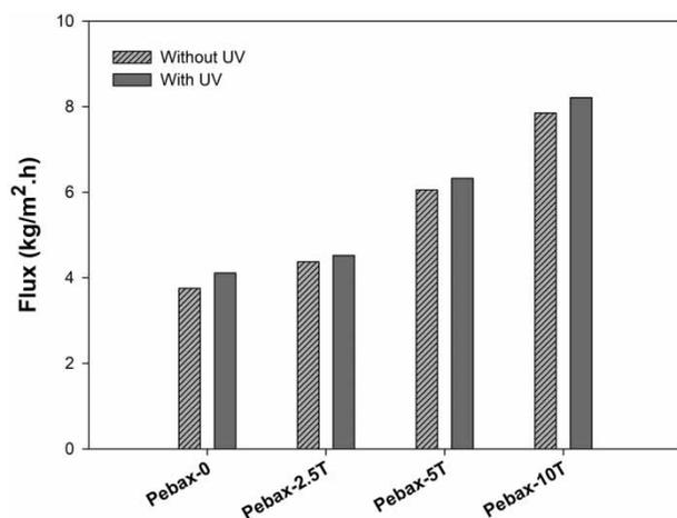
Figure 7 | Flux results of the membranes.
