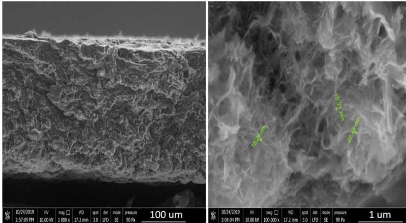
Figure 5 | SEM images of TiO<sub>2</sub>-loaded membranes.
