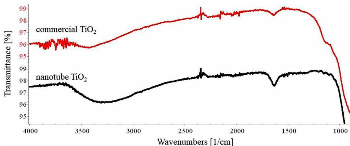
Figure 3 | FTIR spectra of commercial and nanotube  $\text{TiO}_2$ .
