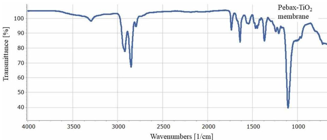
**Figure 2** | FTIR spectra of Pebax- $\text{TiO}_2$  membrane.
