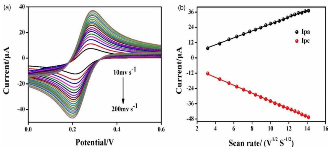
**Figure 3** | (a) Effect of scan rate on the MIP/GCE. The scan rates from inner to outer were 10, 20, 30, 40, 50, 60, 70, 80, 90, 100, 110, 120, 130, 140, 150, 160, 170, 180, 190 and 200  $\text{mVs}^{-1}$ . (b) Plots of the peak currents vs the scan rates in (a).
