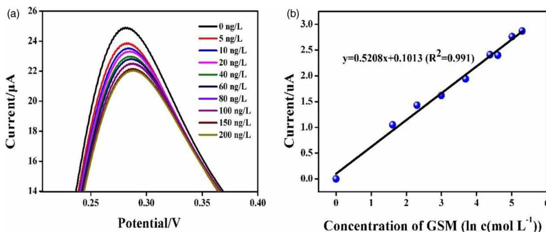
**Figure 5** | (a) CV of the MIP/GCE for 0.2 M pH 5.2 HAC/NaAC containing various concentrations of GSM: 0, 5, 10, 20, 40, 60, 80, 100, 150 and 200 ng L<sup>-1</sup>, respectively. (b) Plots of current versus different GSM concentrations.
