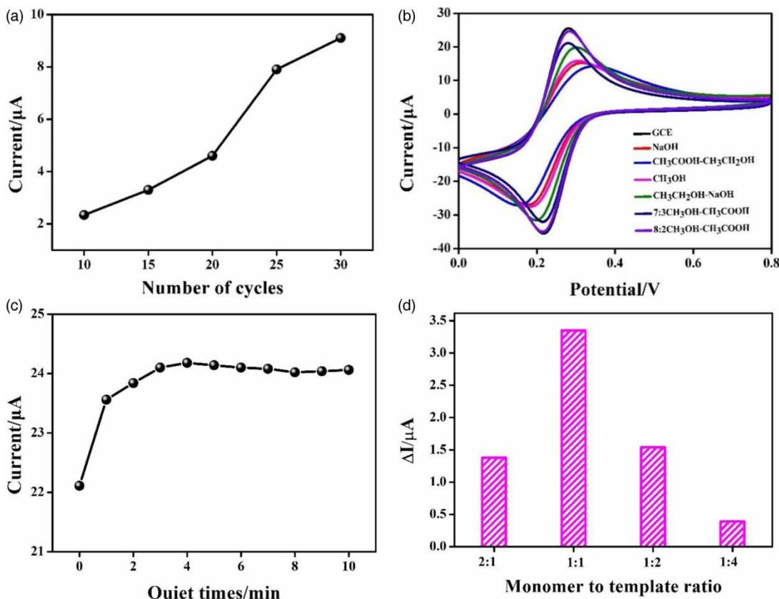
**Figure 4** | (a) Effect of the number of scanning turns on the MIP/GCE electrodes at 10, 15, 20, 25 and 30. (b) Effect of different eluents. (c) Effect of warm bath time. (d) Effect of the ratio between template molecules and monomers.
