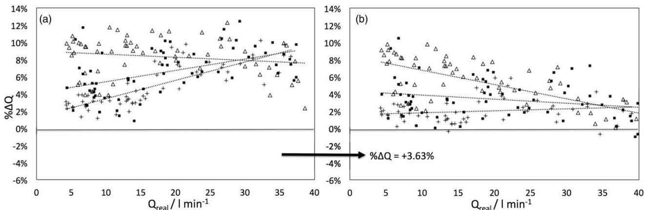
Figure 3 | (a)  $\% \Delta Q$  against  $Q_{\text{real}}$ , disaggregated for flow meters tested; (b) addition of 3.95 s to each measurement in Figure 3(a).
