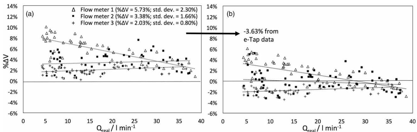
Figure 2 | (a)  $\% \Delta V$  against  $Q_{\text{real}}$ , disaggregated for flow meters tested; (b) reduction of inaccuracies by general calibration of data from Figure 2(a) downwards by  $-3.63\%$ .
