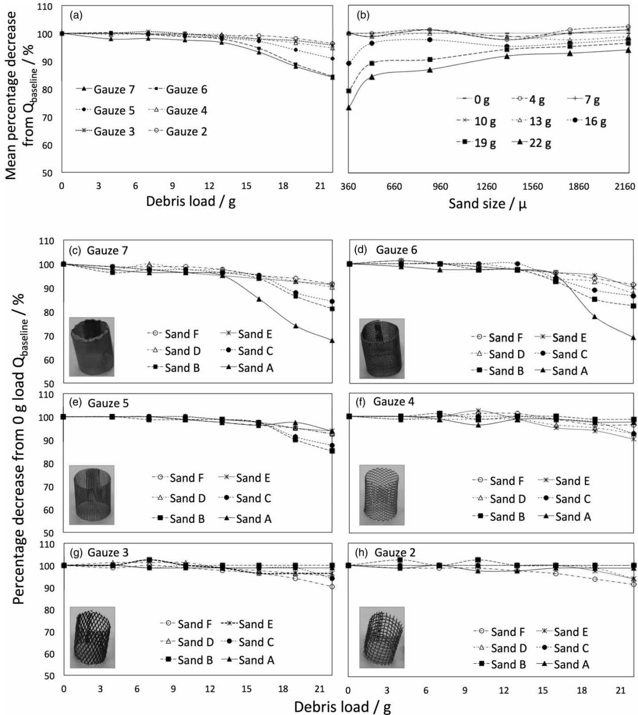
**Figure 4** | (a) Mean percentage  $Q_{baseline}$  decreases over increasing debris loads for each different gauze size, averages for all six sand sizes; (b)  $Q_{baseline}$  decreases for Gauze 7 with increasing debris loads, across varying sand size; (c)–(h) disaggregated  $Q_{baseline}$  decreases per gauze size with varying sand sizes, across increasing debris loads.
