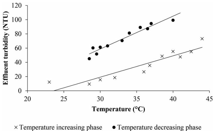
Figure 4 | Variation of effluent turbidity with temperature.
