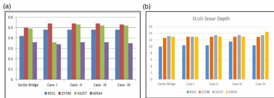
**Figure 10** | (a) Discharge v/s Froude's number for all cases (downstream), (b) Discharge v/s Scour depth for all cases (downstream).
