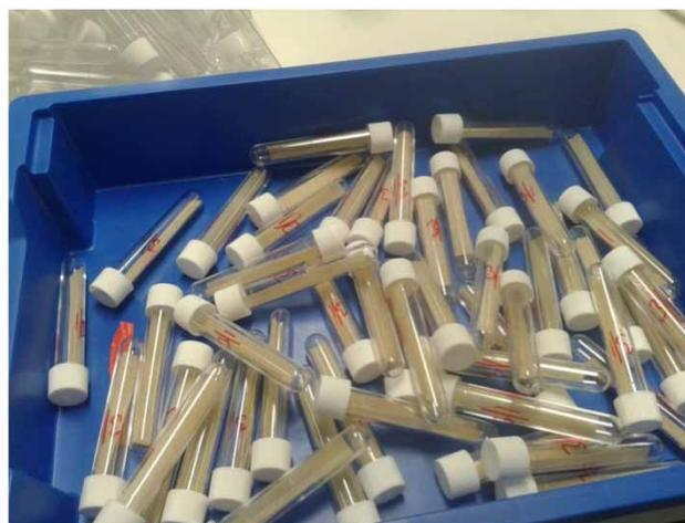
Figure 2 | H<sub>2</sub>S test tubes ready for use.
