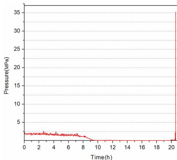
**Figure 9** | Numerical result of pressure at point F for the first accident.
