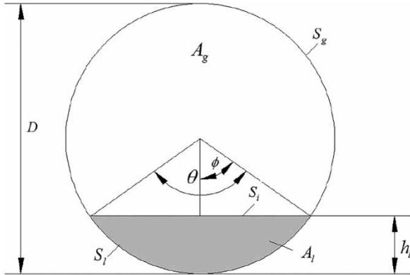
Figure 5 | Geometric relationship of cross-section parameters for stratified flow.
