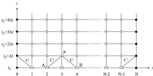
Figure 4 | x-t plane computing grid for difference method. Rectangles: initial points; black dots: boundary nodes; circles: nodes within the boundary.
