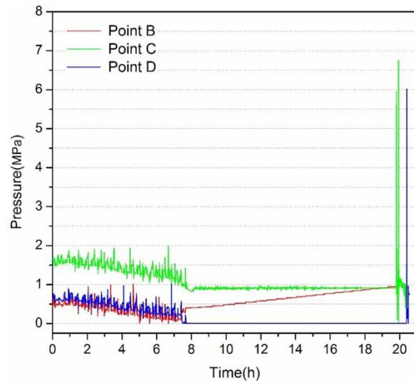
**Figure 8** | Numerical result of pressure at points B, C and D for the first accident.
