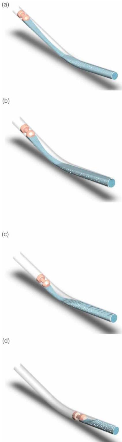
**Figure 3** | Diagram of vapor-liquid eruption: (a) the pig pushes the front air pocket and the liquid column downward at high speed; (b) the front air pocket is connected to the atmosphere; (c) impulse flow; (d) dispersed bubble flow.
