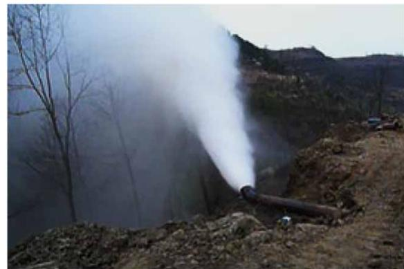
Figure 1 | On-site vapor-liquid flow at the end of a pipeline.
