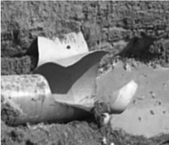
**Figure 2** | The pipe rupture caused by abnormal overpressure (Deng *et al.* 2014).
