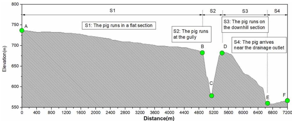
Figure 6 | Elevation profile of pipeline with the first accident.
