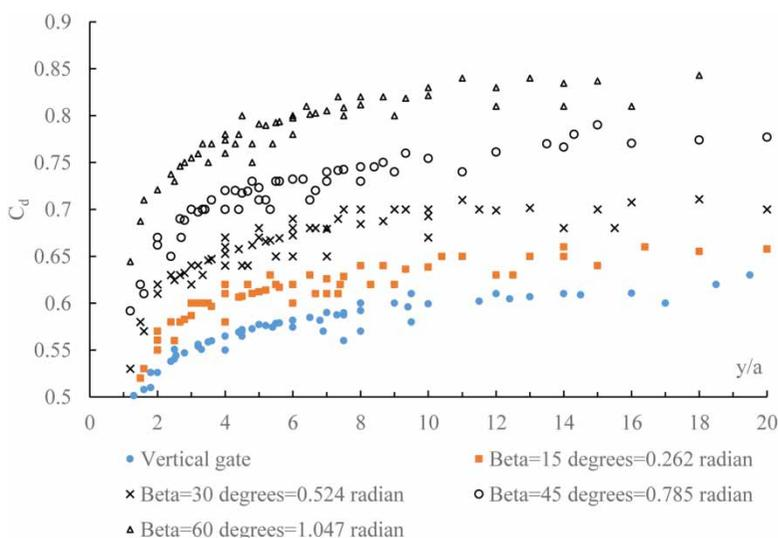
Figure 3 | Inclined gate free flow discharge coefficient variations.
