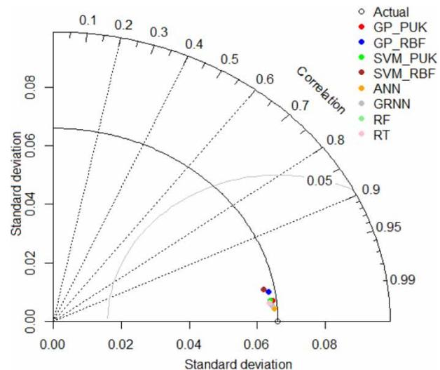
Figure 7 | Taylor plot for comparing the performance of models under free flow conditions. (Figure available in colour on line).
