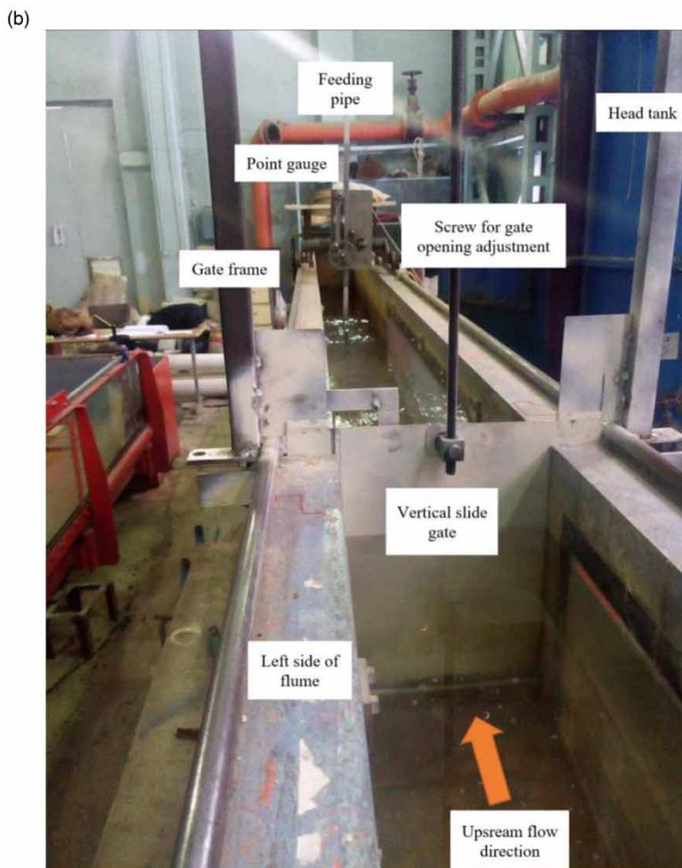
**Figure 2** | The experimental setup. (a) Schematic of experimental setup. (b) Flow in a 10 m flume along with installed vertical gate.
