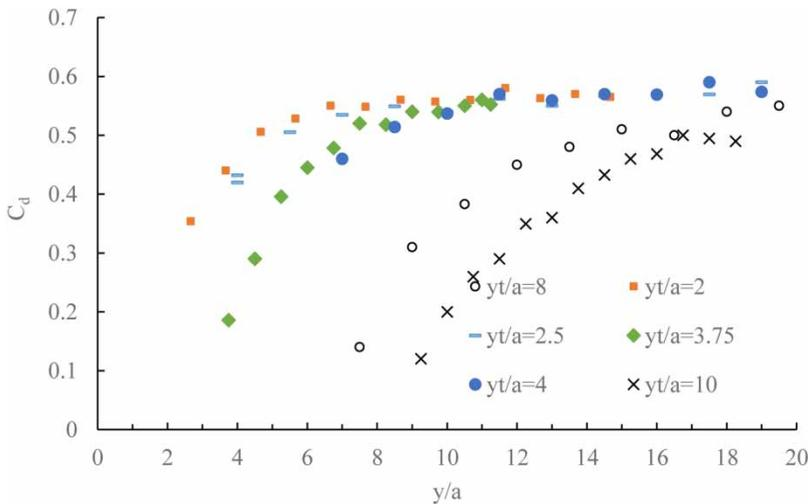
Figure 5 | Submerged inclined gate ( $\beta = 15^\circ$ ) discharge coefficients.
