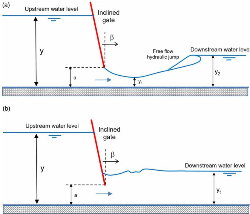
Figure 1 | Free (a) and submerged (b) flow in oblique/inclined sluice gate.
