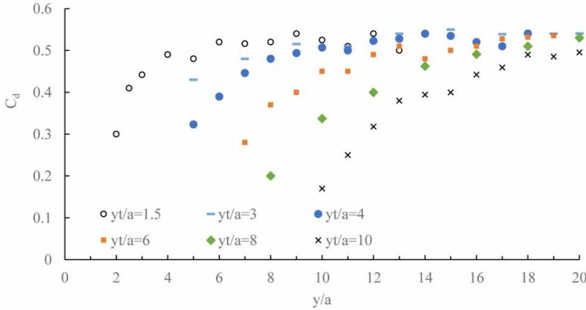
Figure 4 | Submerged vertical gate discharge coefficients.
