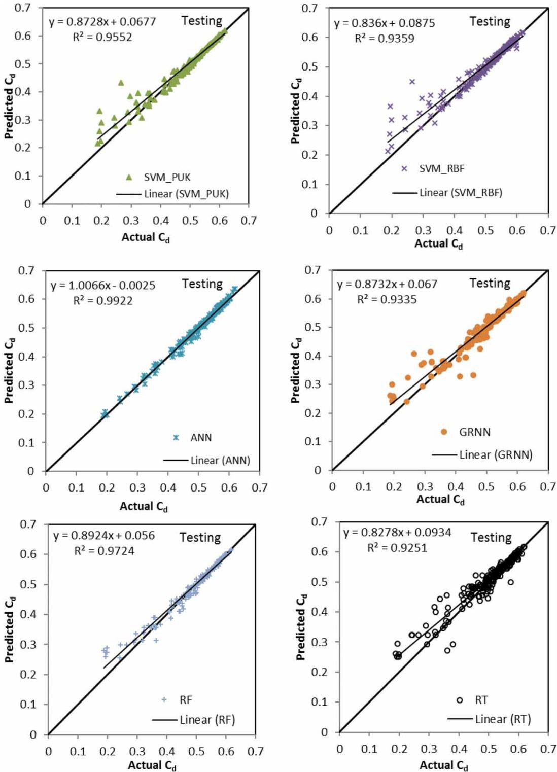
**Figure 8** | Agreement plot for actual and predicted values of  $C_d$  in submerged flow using various soft computing techniques for the testing stage.
