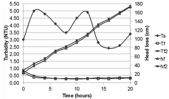
Figure 7 | Influent (settled) and effluent (filtered) water turbidity and total head loss during filtration Run 13;  $T_s$  = settled water turbidity;  $T_f$  = filtered water turbidity (CRS);  $T_{f2}$  = filtered water turbidity (NRS);  $h_f$  = total head loss (CRS);  $h_{f2}$  = total head loss (NRS).
