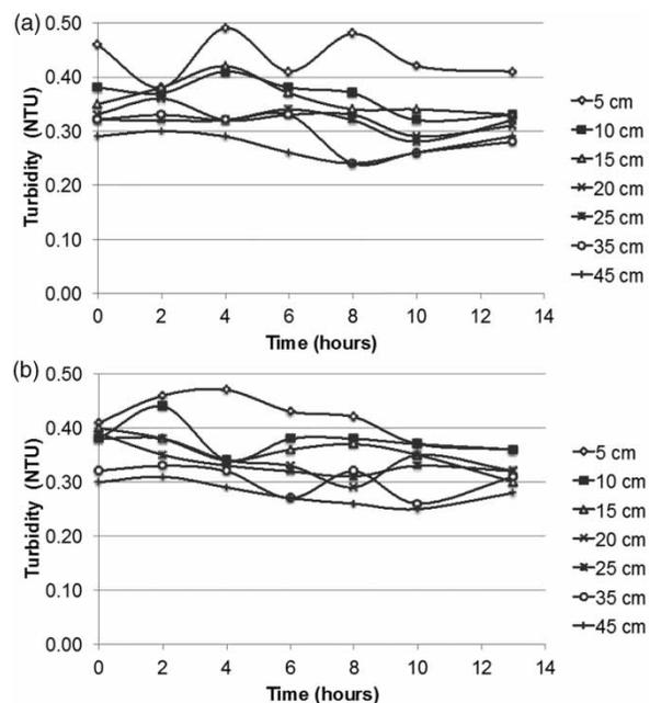
**Figure 2** | Filtered water turbidity during filtration Run 8: (a) CRS filter (b) NRS filter.
