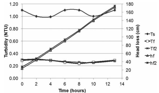
**Figure 4** | Influent (settled) and effluent (filtered) water turbidity and total head loss during filtration Run8. Ts = settled water turbidity; Tf = filtered water turbidity (CRS); Tf<sub>2</sub> = filtered water turbidity (NRS); hf = total head loss (CRS); hf<sub>2</sub> = total head loss (NRS).
