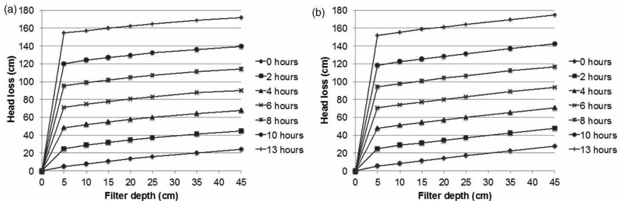
**Figure 3** | Head loss increase along the filter bed depth and over time, filtration Run 8: CRS filter (left) and NRS filter (right).
