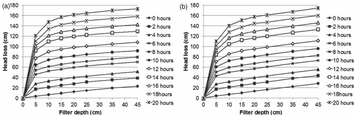
Figure 6 | Head loss increase through the filter bed depth and over time, filtration Run 13: CRS filter (left), NRS filter (right).
