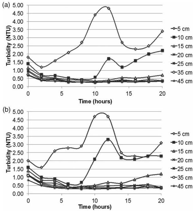
Figure 5 | Filtered water turbidity during filtration Run 13: (a) CRS filter, (b) NRS filter.
