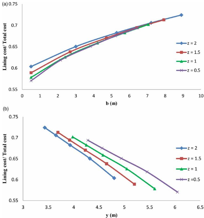
**Figure 4** | Relation between the lining cost/ total cost and (a) the optimal bed width, (b) the optimal water depth for different side slope  $z$ ,  $S.F = 100$ .
