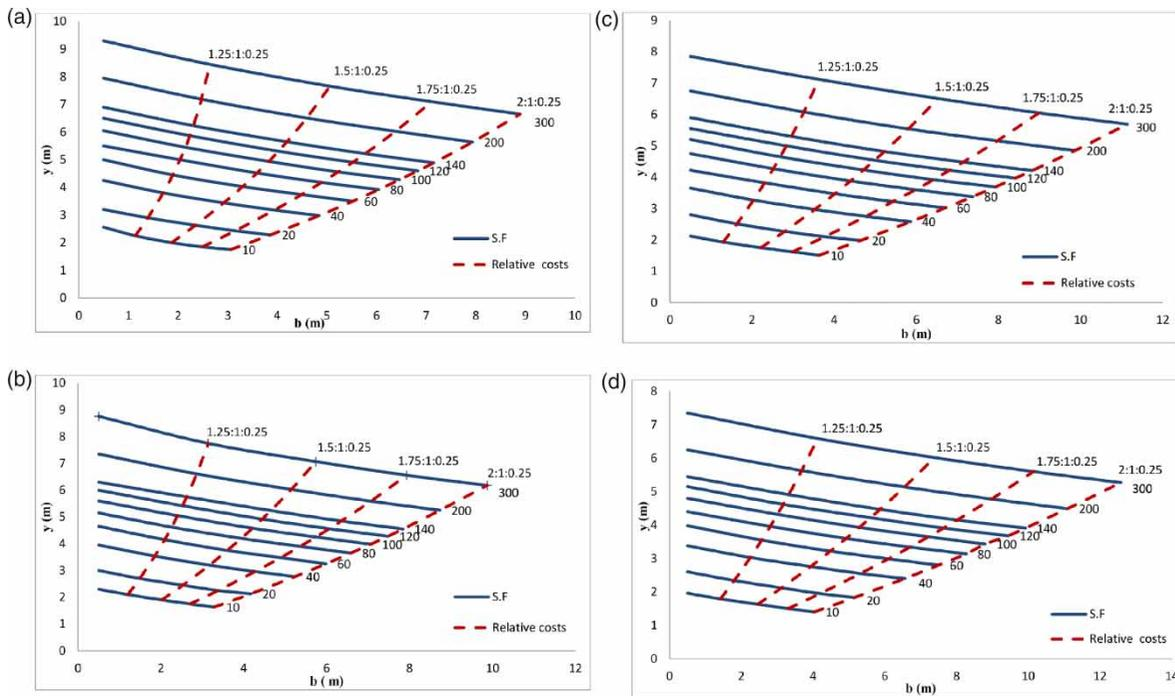
**Figure 3** | Cost minimization design solution ( $l = 0.7$ ). (a)  $Z = 0.5$ . (b)  $Z = 1$ . (c)  $Z = 1.5$ . (d)  $Z = 2$ .
