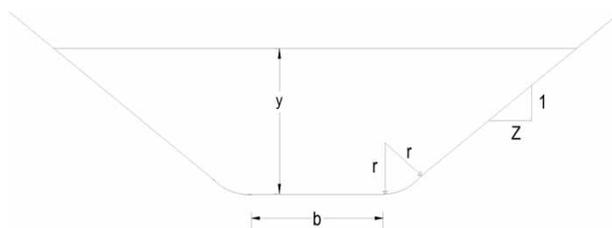
Figure 1 | Definition sketch for the curved corner trapezoidal canal section.
