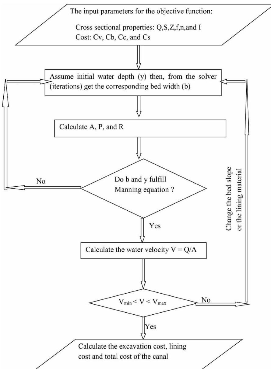
Figure 2 | The optimization model flow chart.
