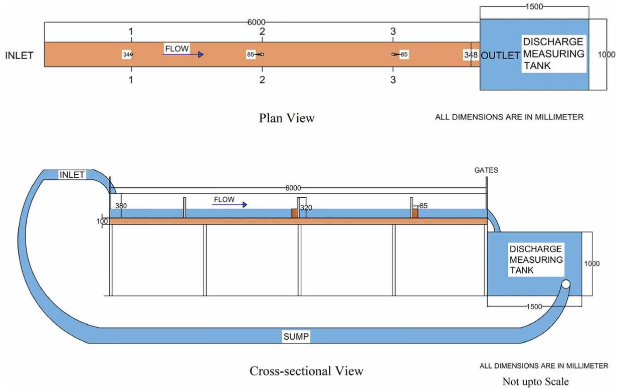
**Figure 3** | Schematic view of experimental setup.
