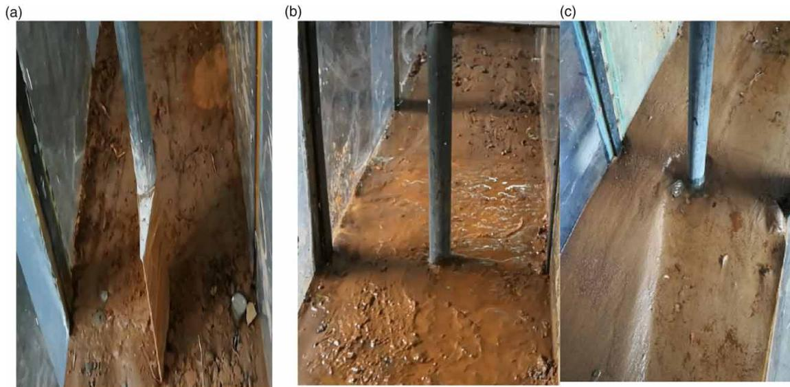
**Figure 4** | (a) Triangular nose on a circular pier, (b) Simple circular pier, (c) Scour action of water on circular pier.
