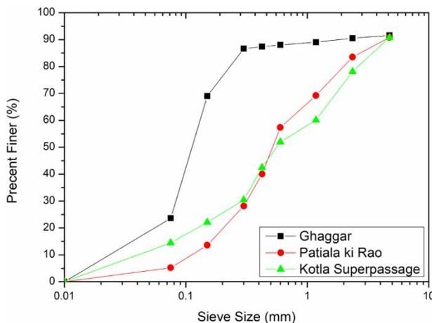
Figure 2 | Grain size distribution curves of soil sample.
