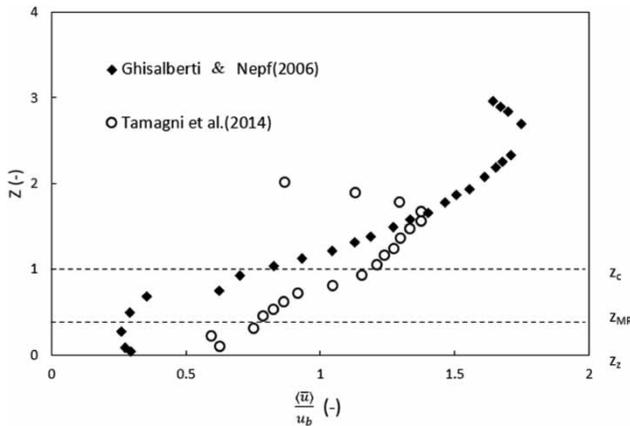
**Figure 9** | Vertical distribution of normalized velocities  $\langle \bar{u} \rangle / u_b$  by Tamagni et al. (2014a, 2014b) and Ghisalberti & Nepf (2006) for  $h_m/p = 1.5$ . where  $u_b$  is the bulk velocity.
