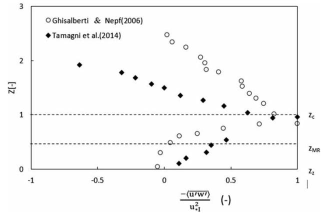
**Figure 10** | Vertical distribution of normalized spatially averaged Reynolds shear stress  $\frac{-\langle \overline{u'w'} \rangle}{u_{*I}^2}$  by Tamagni et al. (2014a, 2014b) and Ghisalberti & Nepf (2006) for  $h_m/p = 1.5$ .
