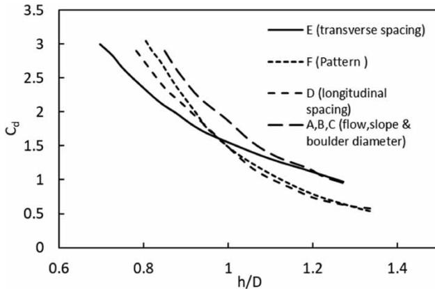
**Figure 12** | Coefficient of drag as a function of submergence ratio  $h/D$  (Baki et al. 2016). Where, A,B,C,D,E and F represents series of varying parameters for flow, slope, boulder diameter, boulder longitudinal spacing, boulder transverse spacing and boulder disposition pattern respectively.
