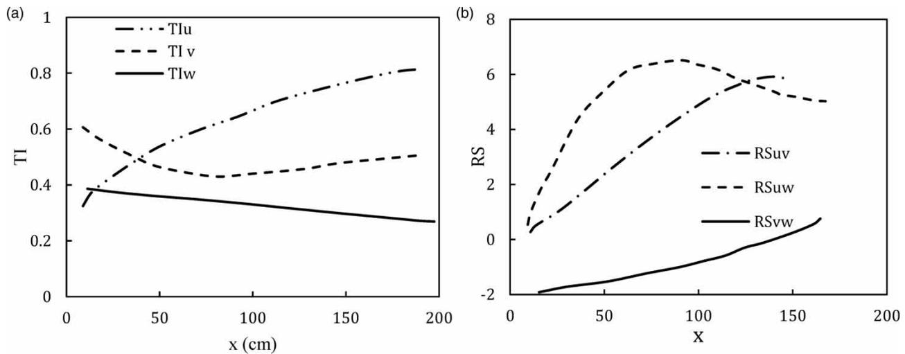
**Figure 7** | (a) Variations of longitudinal  $u'$ , transverse  $v'$  and vertical  $w'$  turbulence intensity along length of ramp (Ahmad *et al.* 2013). (b) Variation of Reynold's Stress along length of block ramp (Ahmad *et al.* 2013).
