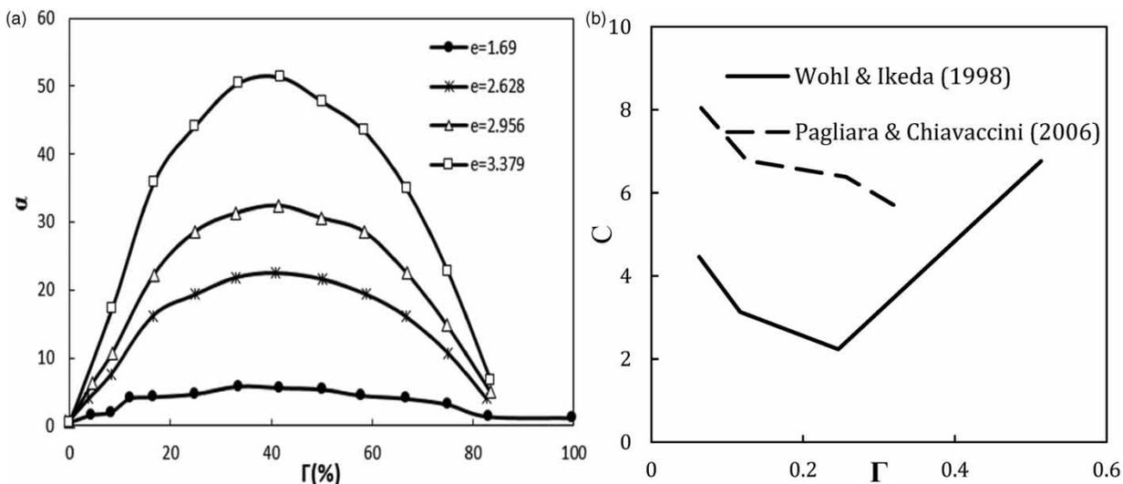
**Figure 2** | (a) Relationship between  $\Gamma$  and  $\alpha$  for given  $e$  ( $=D_{50}/d_{50}$ ) values (Ferro 1999) and (b) Chezy coefficient  $C$  as a function of macroroughness concentration  $\Gamma$  for a transverse row disposition of macroroughness.
