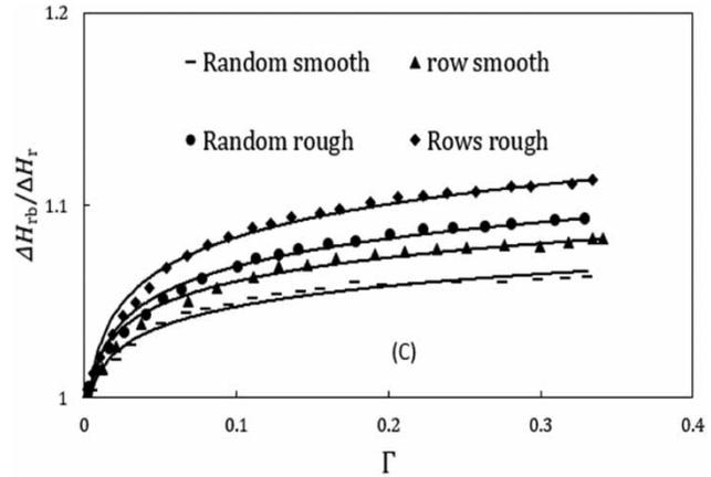
Figure 5 | Shows increase in relative energy dissipation according to Equation (18) for rounded (smooth) and crushed (rough) blocks for different block concentration  $\Gamma$  (Pagliara & Chivaccini 2006b).
