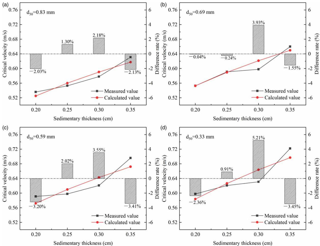
**Figure 5** | Comparison between the calculated and the measured values of the critical velocity for steel/PVC pipe. (a)  $d_{50} = 0.83$  mm; (b)  $d_{50} = 0.69$  mm; (c)  $d_{50} = 0.59$  mm; (d)  $d_{50} = 0.33$  mm.
