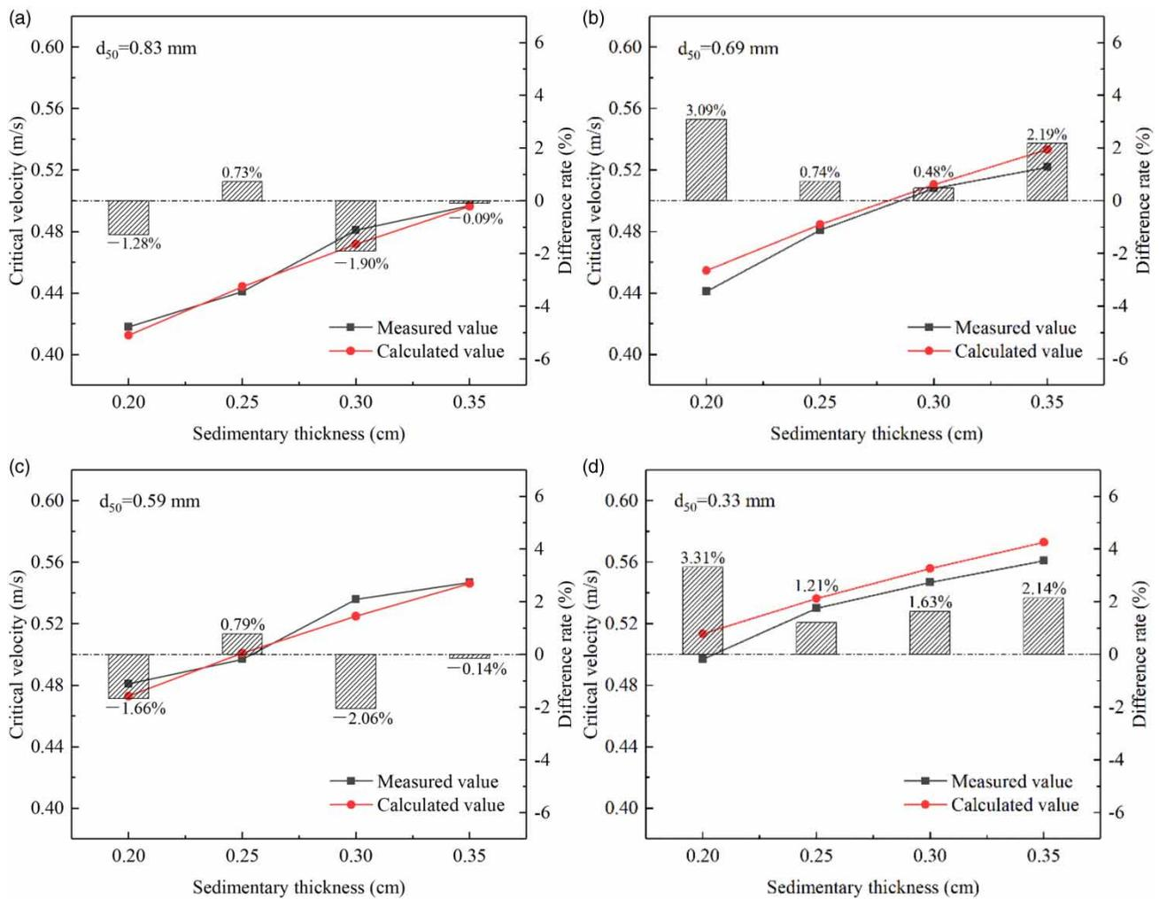
**Figure 4** | Comparison between the calculated and the measured values of the critical velocity for plexiglass pipe. (a)  $d_{50} = 0.83$  mm; (b)  $d_{50} = 0.69$  mm; (c)  $d_{50} = 0.59$  mm; (d)  $d_{50} = 0.33$  mm.
