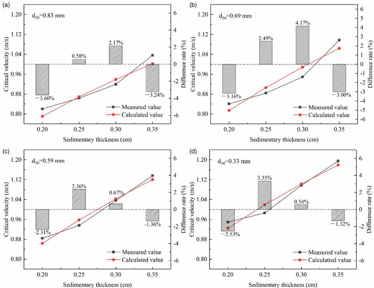
**Figure 7** | Comparison between the calculated and the measured values of the critical velocity for cast iron pipe. (a)  $d_{50} = 0.83$  mm; (b)  $d_{50} = 0.69$  mm; (c)  $d_{50} = 0.59$  mm; (d)  $d_{50} = 0.33$  mm.
