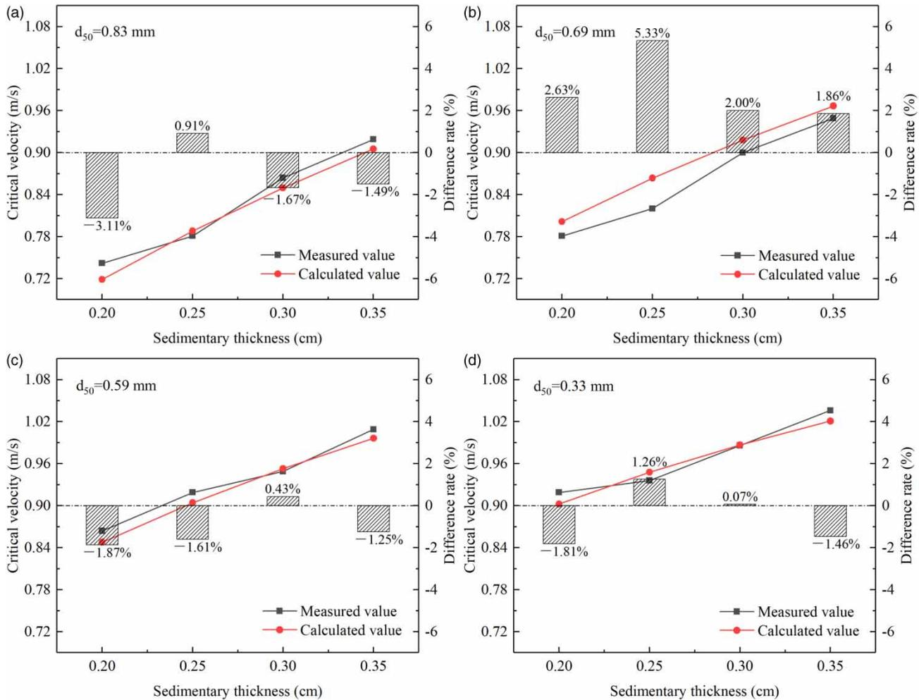
**Figure 6** | Comparison between the calculated and the measured values of the critical velocity for galvanized/clay pipe. (a)  $d_{50} = 0.83$  mm; (b)  $d_{50} = 0.69$  mm; (c)  $d_{50} = 0.59$  mm; (d)  $d_{50} = 0.33$  mm.
