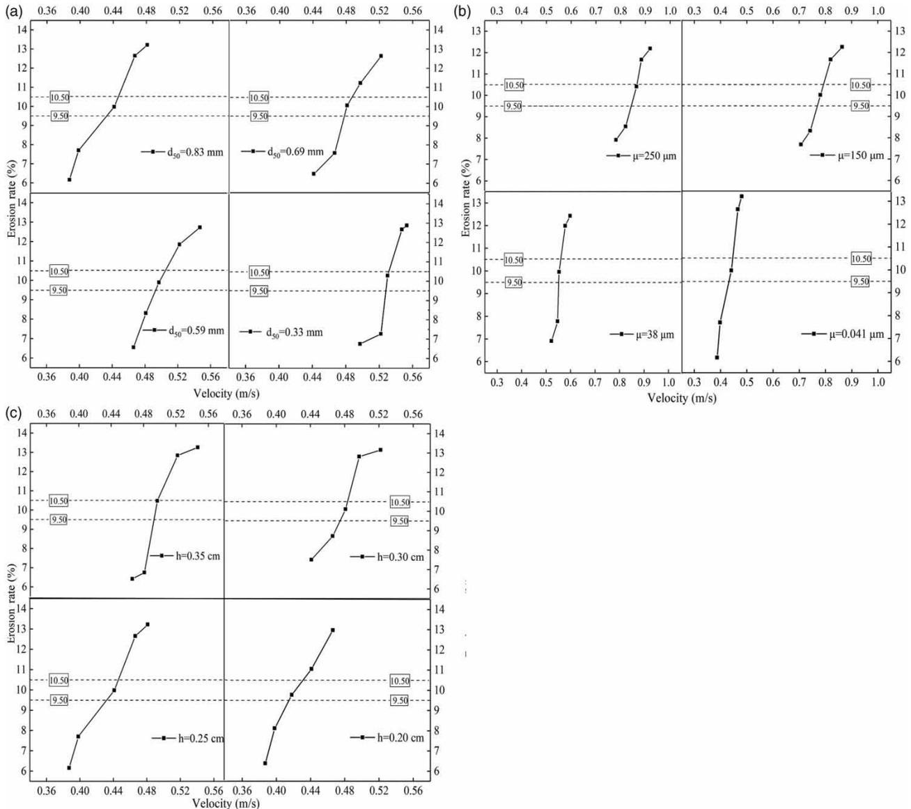
**Figure 2** | Influencing factors of the migration critical velocity. (a) Sediment particle size ( $\mu = 0.041 \mu\text{m}$ ,  $h = 0.25 \text{ cm}$ ); (b) pipe wall roughness ( $d_{50} = 0.83 \text{ mm}$ ,  $h = 0.25 \text{ cm}$ ); (c) sediment thickness ( $d_{50} = 0.83 \text{ mm}$ ,  $\mu = 0.041 \mu\text{m}$ ).
