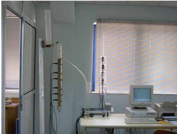
Figure 1 | The first experimental setting. (cumulative infiltration with ~2 mm head boundary condition).
