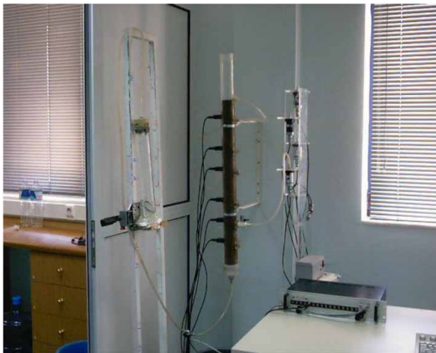
Figure 2 | The second experimental setting (upward infiltration).
