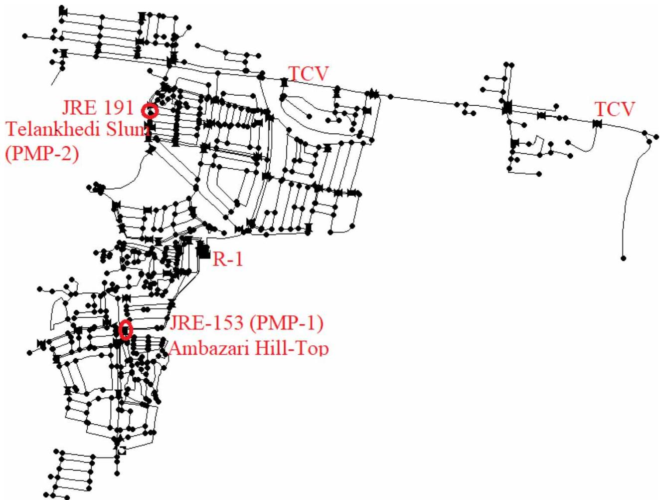
**Figure 1** | Layout of water distribution network of Ramnagar ESR Nagpur, Maharashtra, India, consisting of 69 TCV (EPANET Model).
