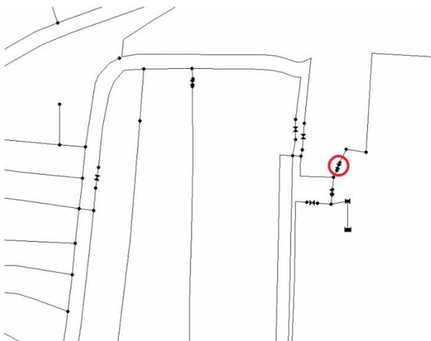
**Figure 2** | TCV in ESR premises in EPANET model, which are operated at different times in a day.
