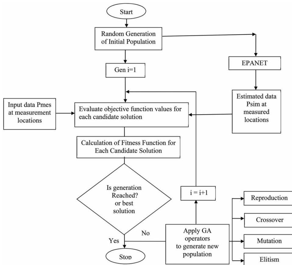
Figure 3 | Flow chart of hydraulic calibration model using GA.
