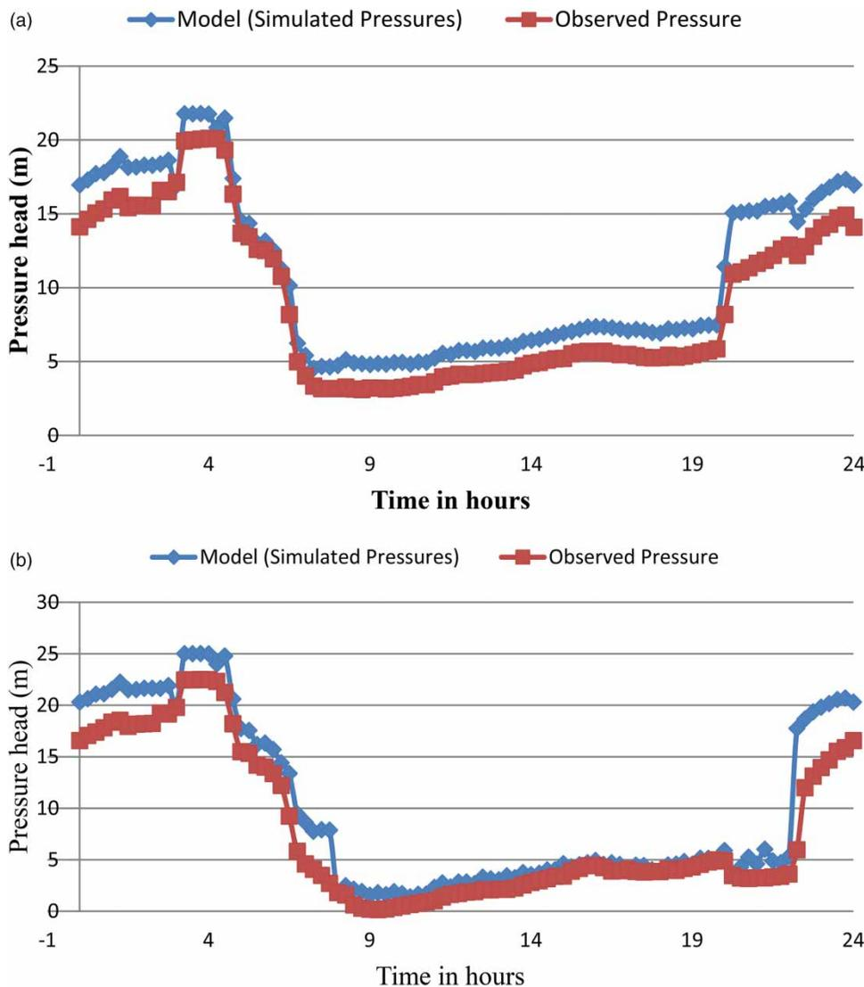
**Figure 4** | Comparison of computed/simulated pressure with observed pressure at both CPs. (a) Ambazari Hill-Top Slum (PMP-1/CP1) (b) Telankhedi Slum (PMP-2/CP2).
