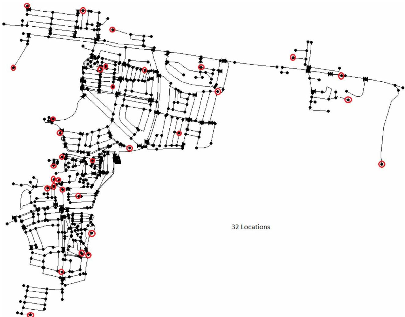
Figure 6 | Location of 32 optimal sensor locations on calibrated zone of case study.
