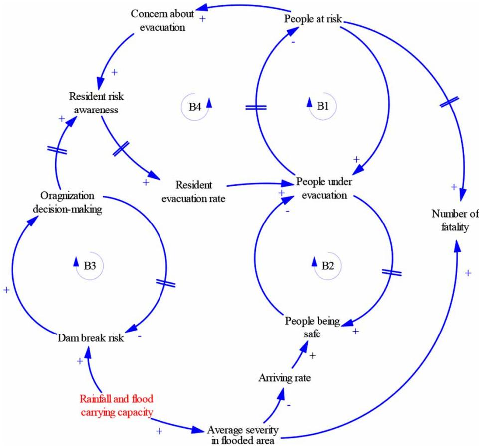
Figure 7 | Completed causality model of reservoir dam break risk dynamics (only the critical variables are shown).
