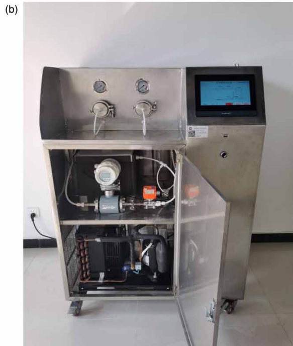
Figure 1 | (a) Diagram of the integrated membrane performance testing device. (b) Image of the integrated membrane performance testing device.
