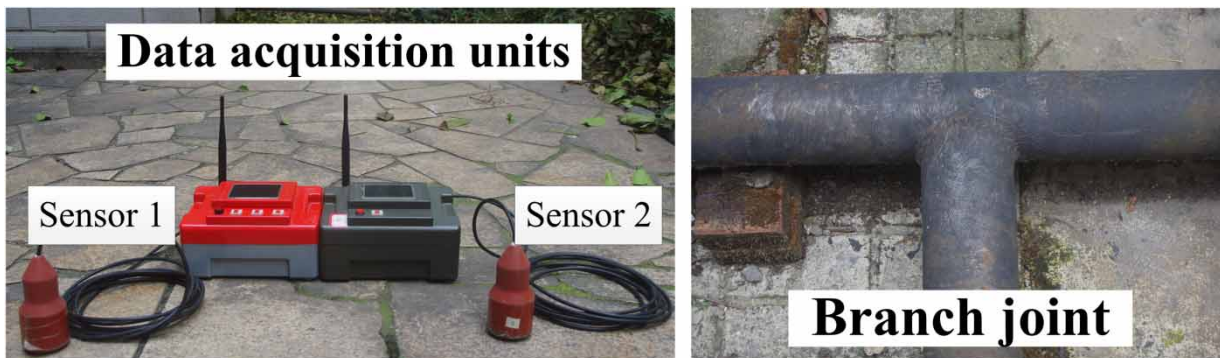
Figure 7 | Pictures of branch joint, Sensor 1 and Sensor 2.
