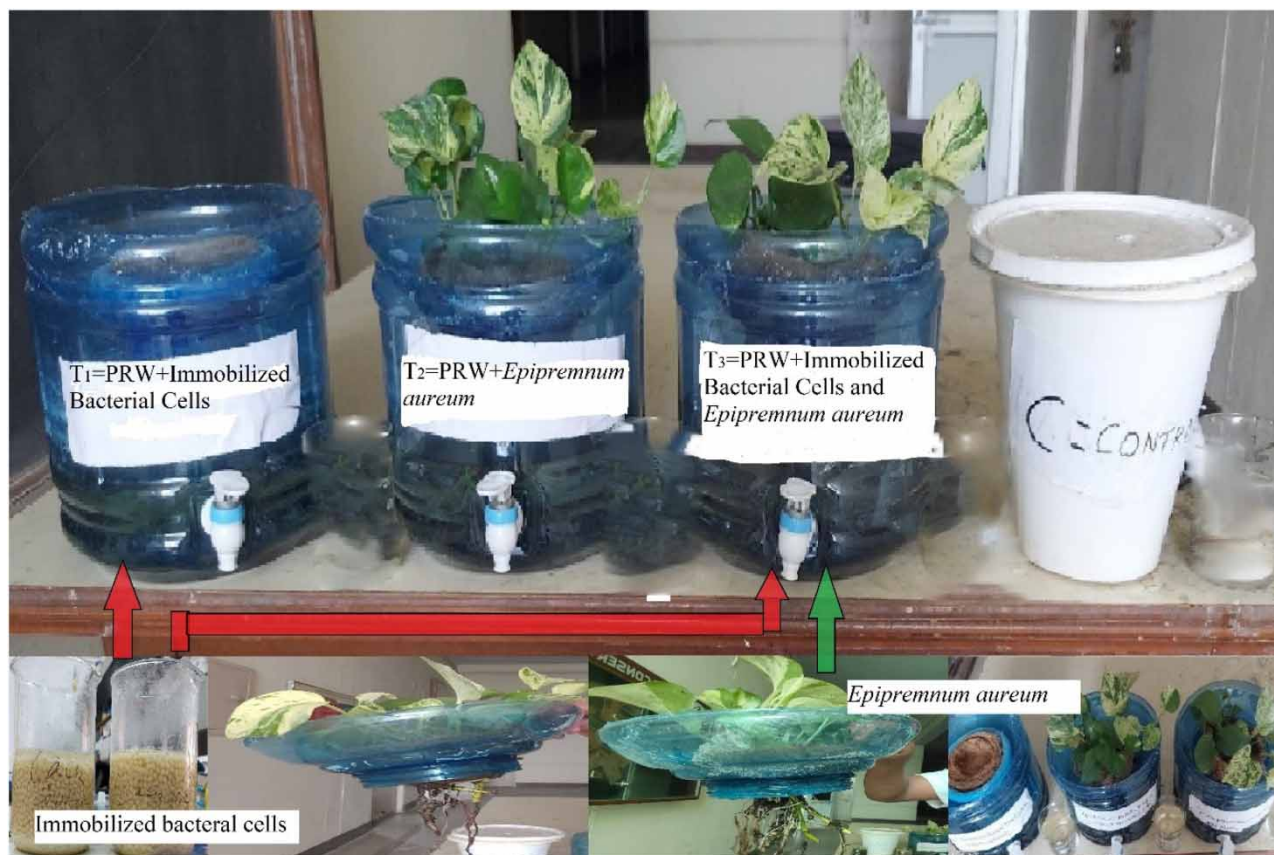
Figure 2 | Experimental setups for treatment of polluted river water.
