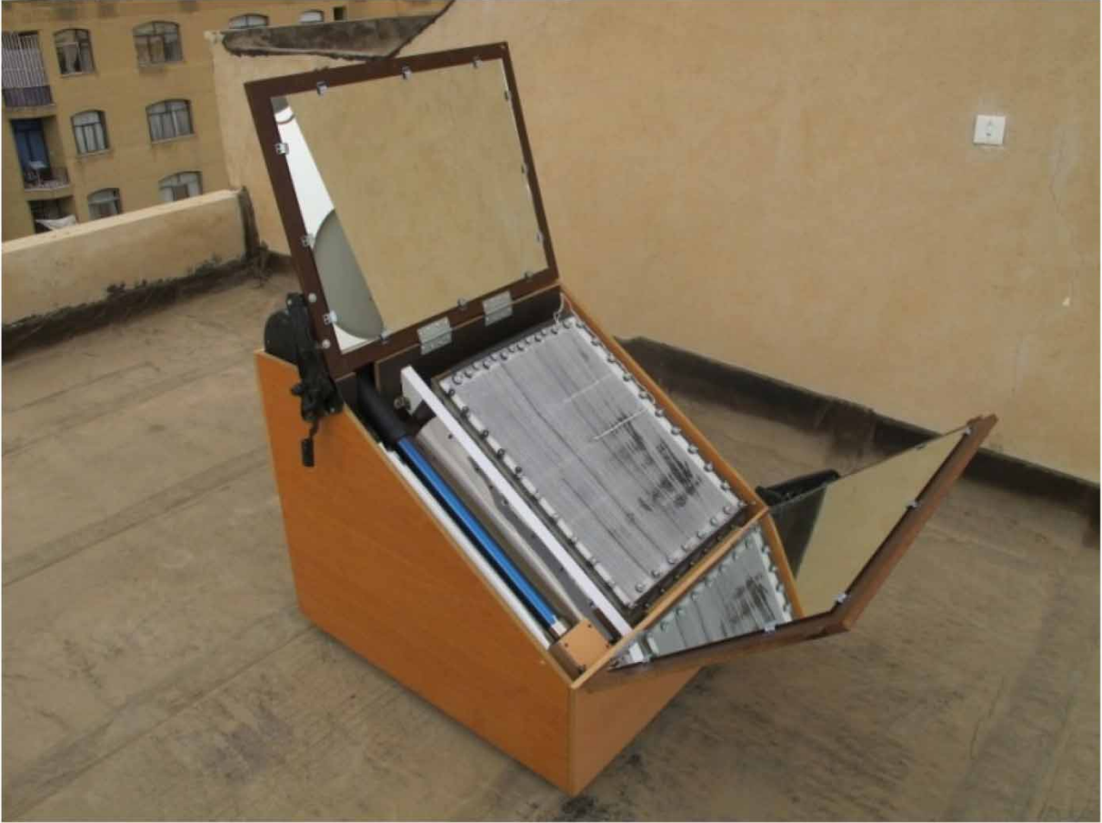
Figure 3 | A view of the solar still system manufactured and tested in this research.
