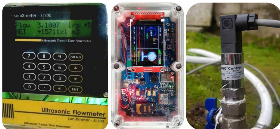
Figure 8 | The installed flowmeter, pressure sensor and data loggers.
