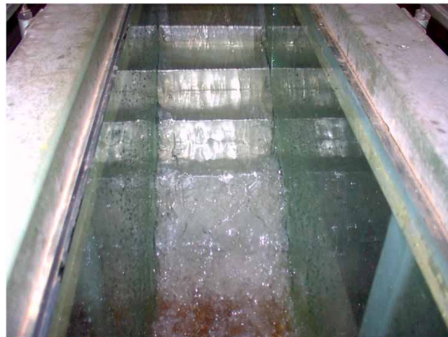
Figure 6 | Flow over stepped spillway (downstream view).
