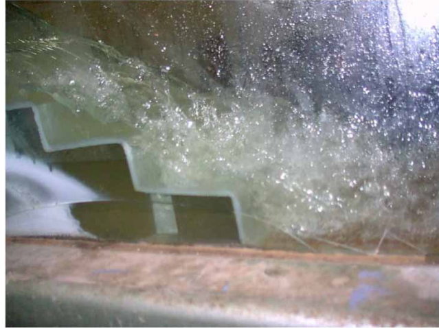
Figure 7 | Close-up of flow over stepped spillway (side view), turbulent and energy dissipation at the toe of the spillway (Salmasi & Samadi 2018).
