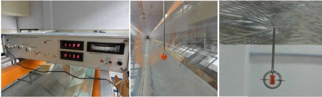
Figure 2 | Propeller velocity flowmeter (Armfield 3000 mm/s – H32-1A model).
