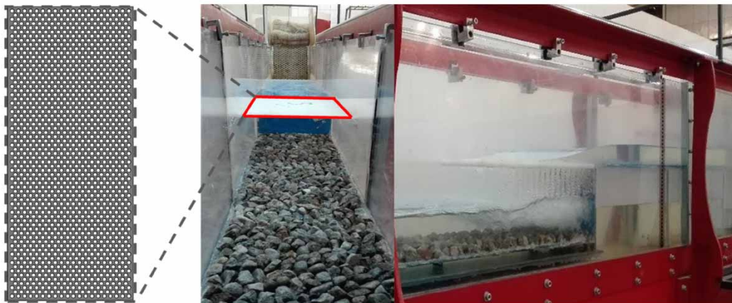
Figure 3 | Schematic of the laboratory model on rough bed.
