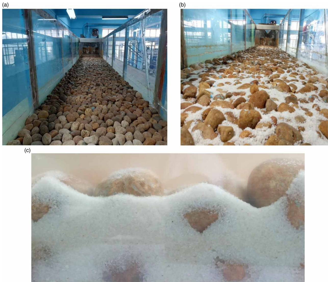
Figure 1 | Photographs of the experimental setup: (a) long section of a gravel bed, (b) long section of a sand-filled gravel bed and (c) side view of the sand-fill process.
