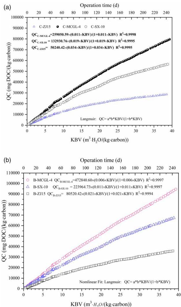
**Figure 6** | Cumulative uptake of DOC and related parameters. (a) Pilot-scale BAC system; (b) Pilot-scale BEAC system.
