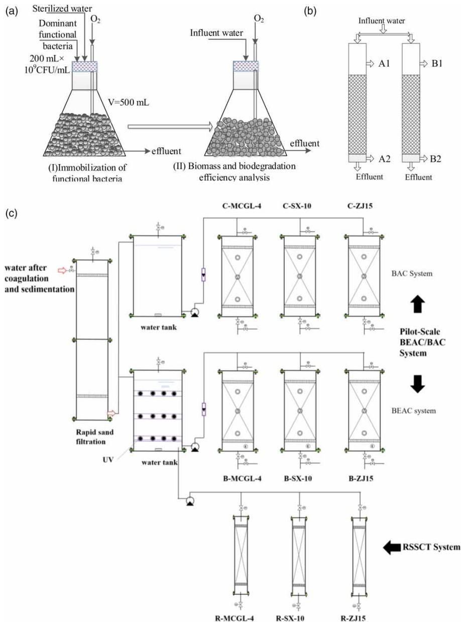
**Figure 2** | Experimental set-up. (a) Evaluation set-up for initially immobilized biomass, (b) evaluation set-up for dissolved oxygen utilization, (c) pilot-scale BEAC/BAC system and RSSCT tests system.
