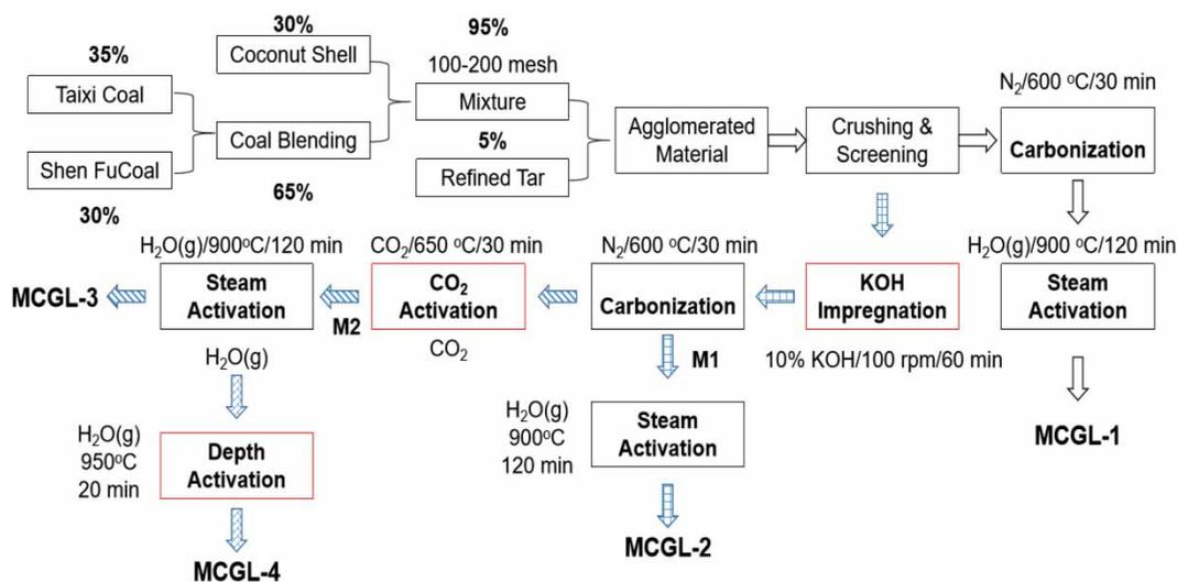
**Figure 1** | Preparation procedure of new carbons.
