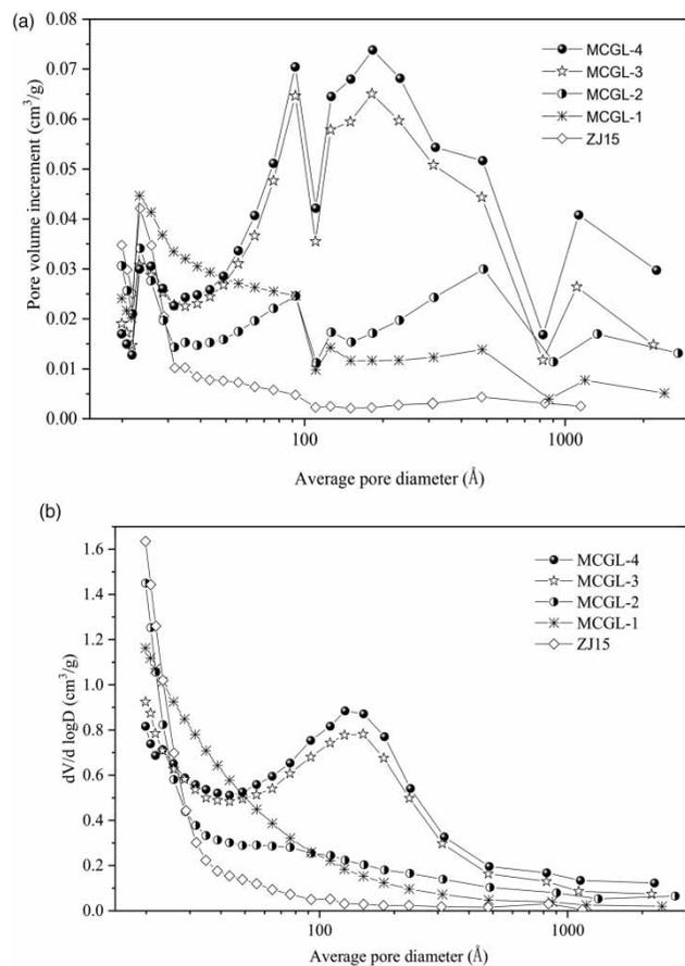
**Figure 3** | Physico-chemical properties of new carbons. (a) Distribution of pore size and pore volumes, (b) dV/d logD.
