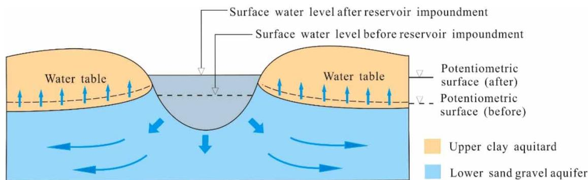
Figure 1 | Schematic diagram of immersion process in dual-formation structural reservoir bank.
