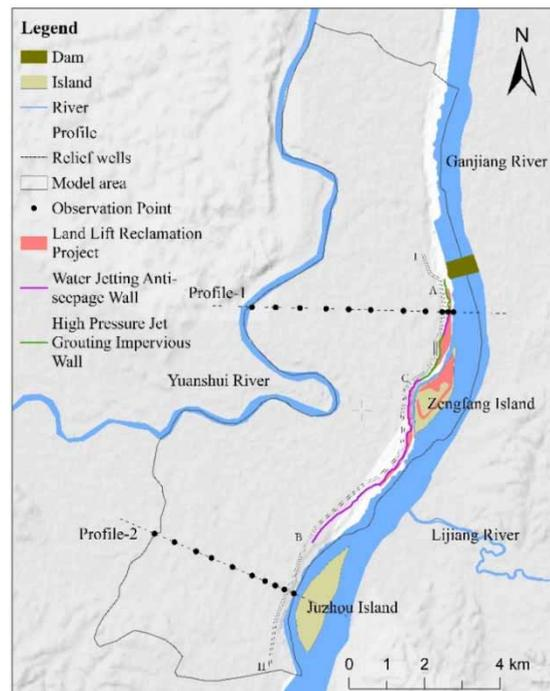
**Figure 9** | Layout of engineering measures including cut-off walls, relief wells, and land lift reclamation for controlling reservoir immersion.
