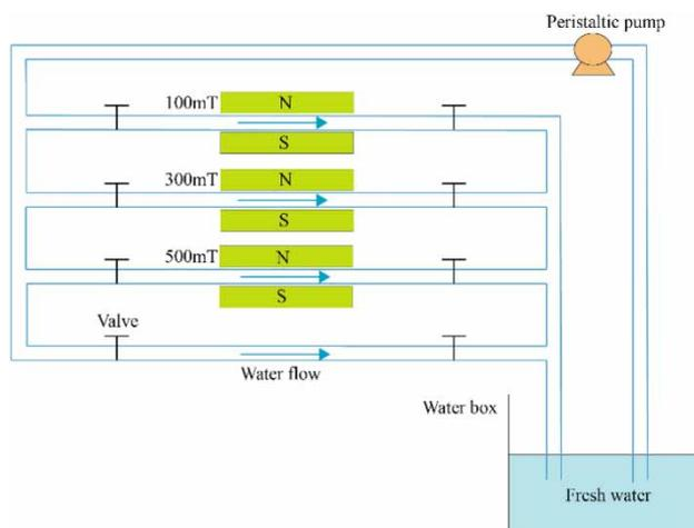
Figure 1 | Schematic diagram of magnetized water device.
