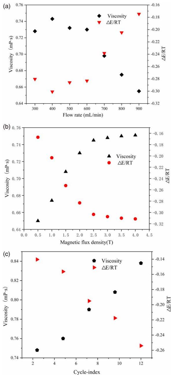
**Figure 3** | The effect of (a) flow rate, (b) magnetic flux density and (c) cycle-index on viscosity.
