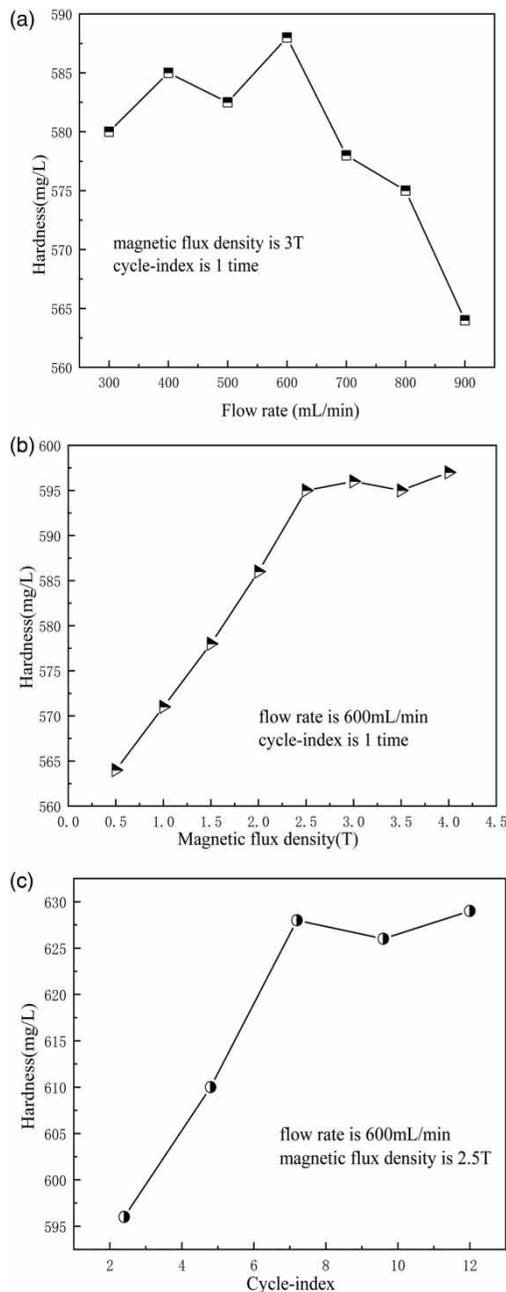
**Figure 2** | The influence of (a) flow rate, (b) magnetic flux density and (c) cycle-index on association solubilization.
