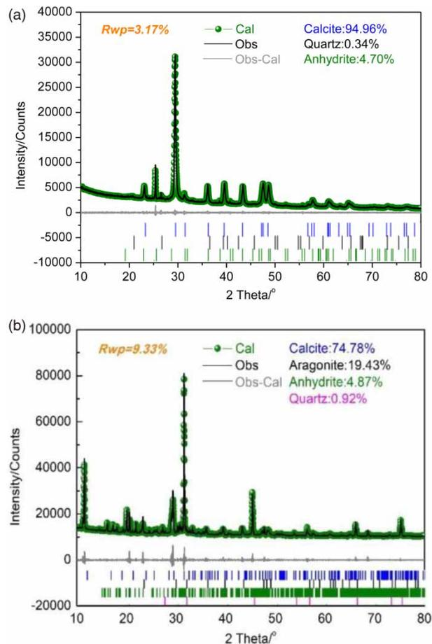
Figure 5 | XRD analysis of scale in untreated (a) and treated (b) by S-HGMF.
