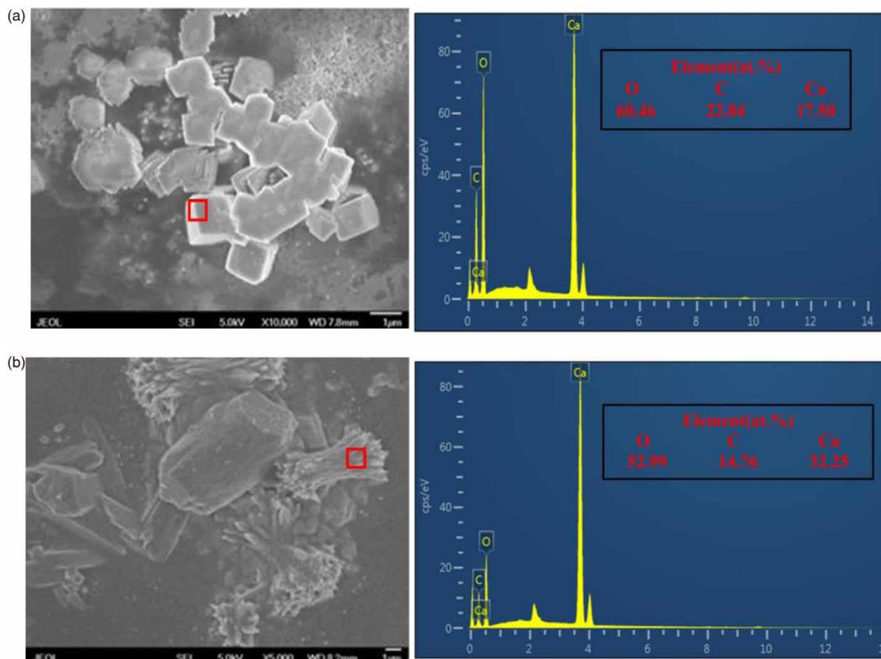
**Figure 6** | SEM analysis of scale in untreated (a) and Treated (b) by S-HGMF.
