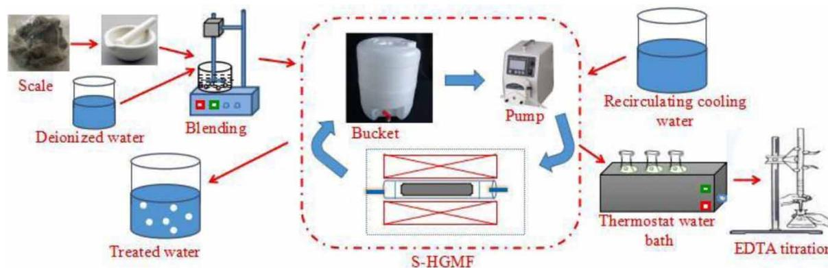
Figure 1 | Experimental flow chart of S-HGMF treatment.
