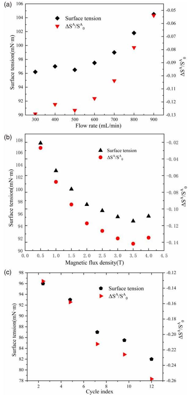
Figure 4 | The effect of (a) flow rate, (b) magnetic flux density and (c) cycle-index on surface tension.
