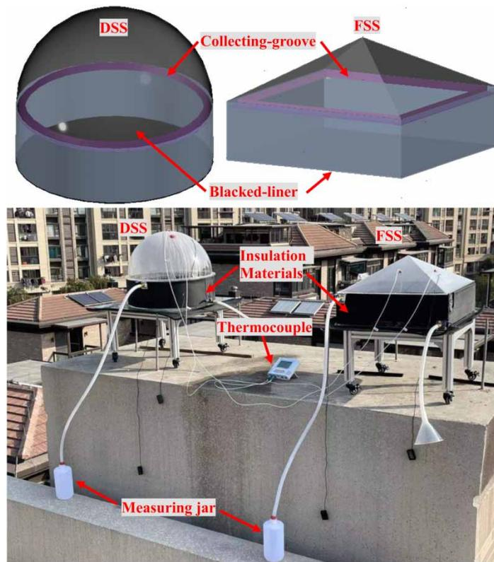
**Figure 1** | Photograph of experimental test rig of FSS and DSS.
