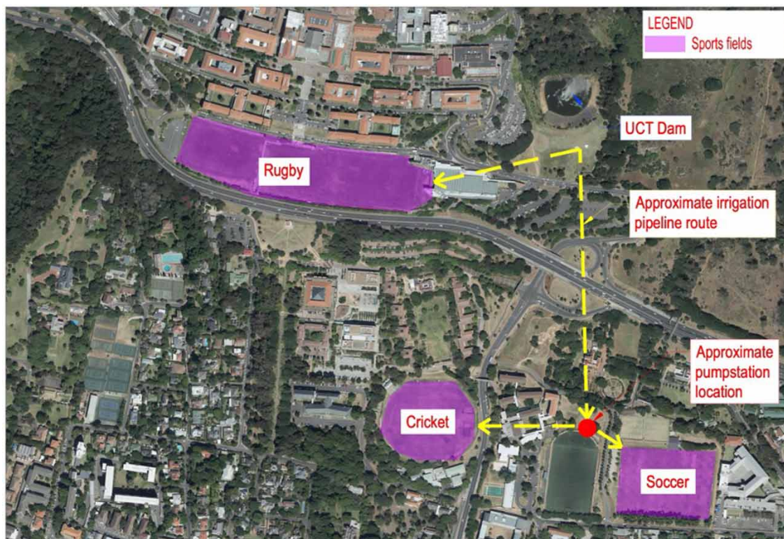
Figure 4 | Proposed irrigation pipeline routes and pump station location (adapted with permission from Zutari 2020).
