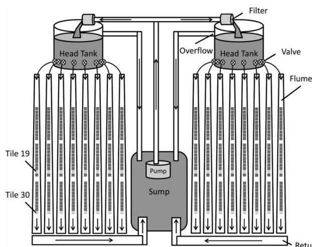
Figure 1 | Replicated flowways ( $n = 16$ ) used in these algal treatment system experiments.
