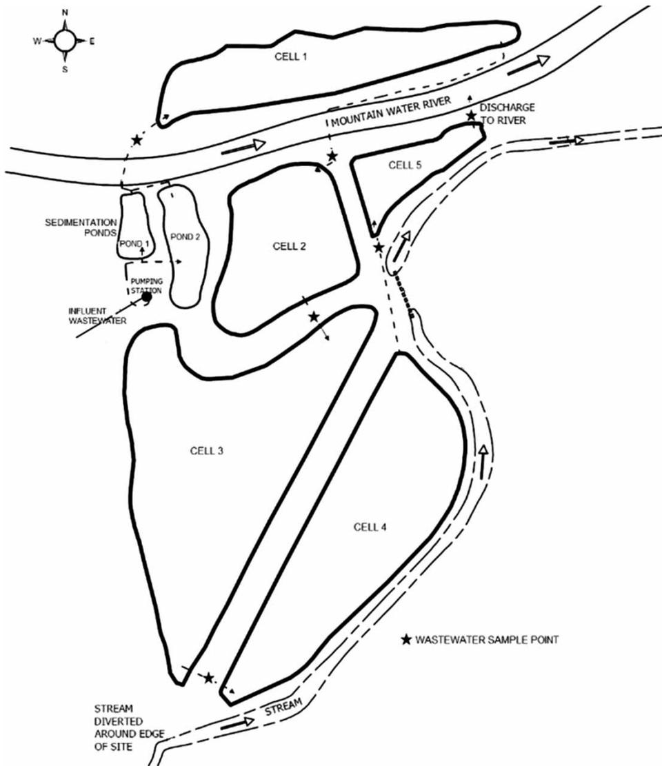
Figure 1 | Schematic diagram of integrated constructed wetland at Glaslough in Ireland.
