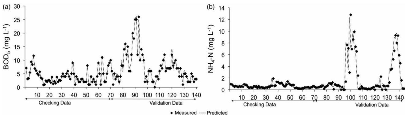
Figure 4 | Performance of ANFIS models in predicting (a)  $BOD_5$  and (b)  $NH_4-N$  in ICW effluent.
