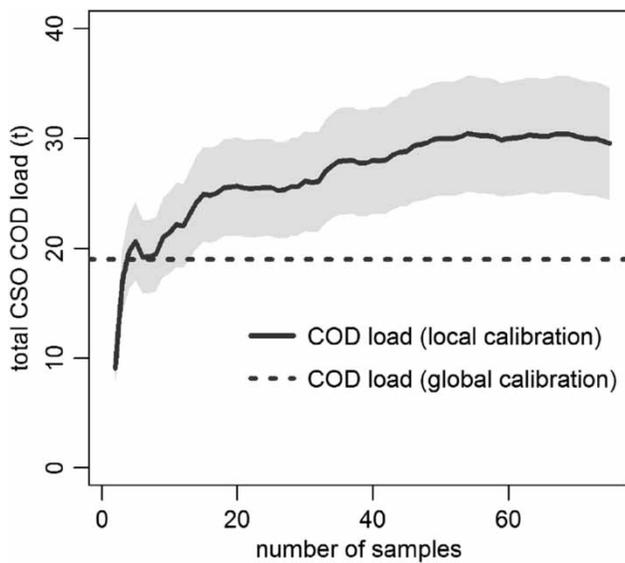
**Figure 4** | Influence of the number of samples on total COD load calculated using local and global calibration functions in Berlin.
