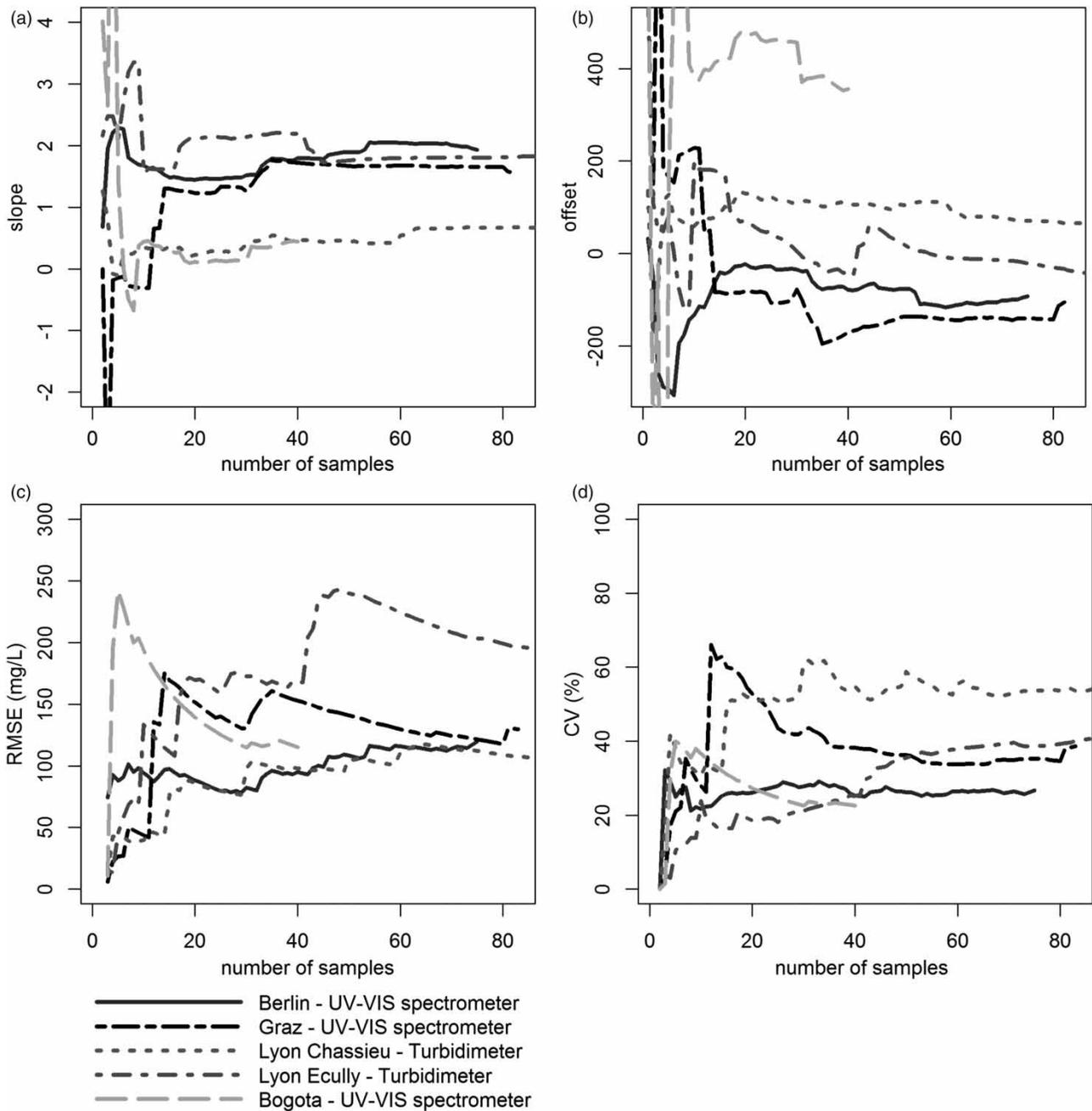
**Figure 3** | Influence of the number of samples used to establish calibration functions in each study site.
