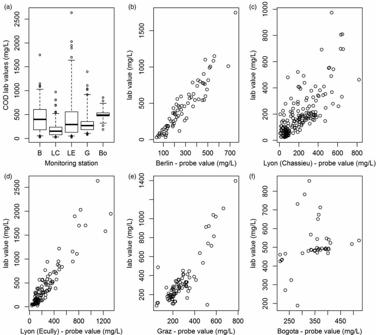
**Figure 2** | (a) The box plots of laboratory values obtained during rain events in each case study: B for Berlin, LC for Lyon Chassieu, LE for Lyon Ecully, G for Graz and Bo for Bogota. (b)–(f) The pairs of probe values and related COD laboratory values of samples collected at the times of the probe measurements.
