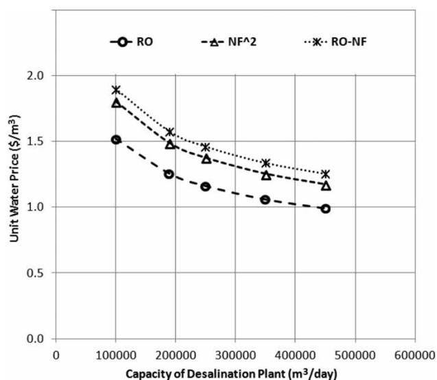
**Figure 3** | Comparison of unit water price for RO, NF<sup>2</sup>, RO-NF desalination facilities;  $i$ : 10%; lifetime: 25 years; costs: 2013 USD; design flow rate to average flow rate ratio = 1.3.
