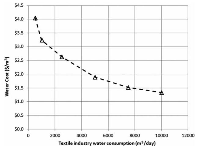
**Figure 4** | Unit reused water cost for dye-bath effluent treatment by UF-NF system ( $\epsilon$ : 10%; lifetime: 25 years; costs: 2013 USD; design flow rate to average flow rate ratio = 2).
