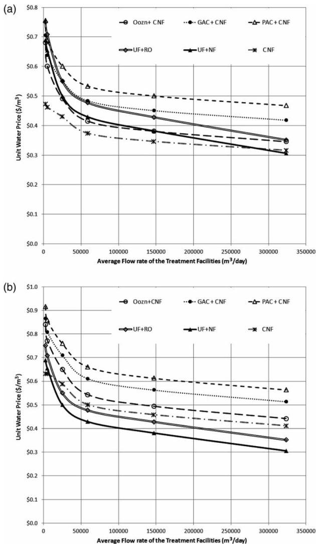
**Figure 2** | Unit cost (\$/m<sup>3</sup>) for tertiary treated wastewater for indirect potable water applications; *i*:10%; lifetime: 25 years; costs: 2013 USD; A: CNF/NF cost = 5, B: CNF/NF cost = 15; design flow rate to average flow rate ratio = 1.7 for capacity > 50,000 m<sup>3</sup>/day and 2 for capacities ≤ 50,000 m<sup>3</sup>/day.
