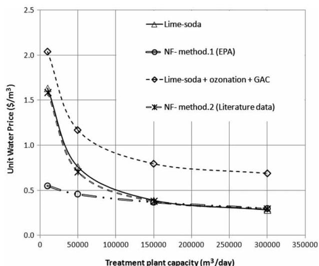
**Figure 1** | Water cost for water softening and color removal alternatives;  $i$ : 10%; lifetime: 25 years; costs: 2013 USD; design flow rate to average flow rate ratio = 1.7 for capacity > 50,000 m<sup>3</sup>/day and 2 for capacities ≤ 50,000 m<sup>3</sup>/day.
