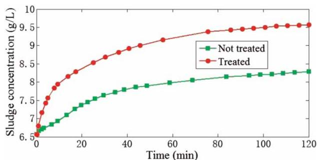
Figure 4 | Effect of denitrification on sludge thickening ('treated' refers to the experiment without denitrification, and 'not treated' refers to the experiment with denitrification).
