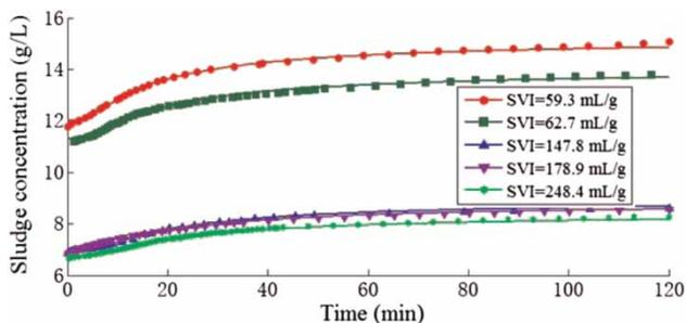
Figure 2 | Five sludge-thickening curves in the compression zone.
