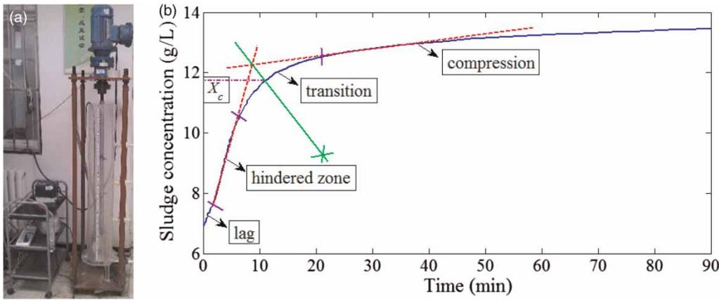
Figure 1 | (a) Schematic diagram of experimental set-up, and (b) example-thickening curve for the activated sludge.
