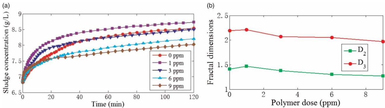
**Figure 5** | (a) Activated sludge thickening, and (b)  $D_2$  and  $D_3$  for sludge flocs with different cationic PAM doses ( $D_2$  and  $D_3$  refer to the two- and three-fractal dimensions of the floc, respectively).
