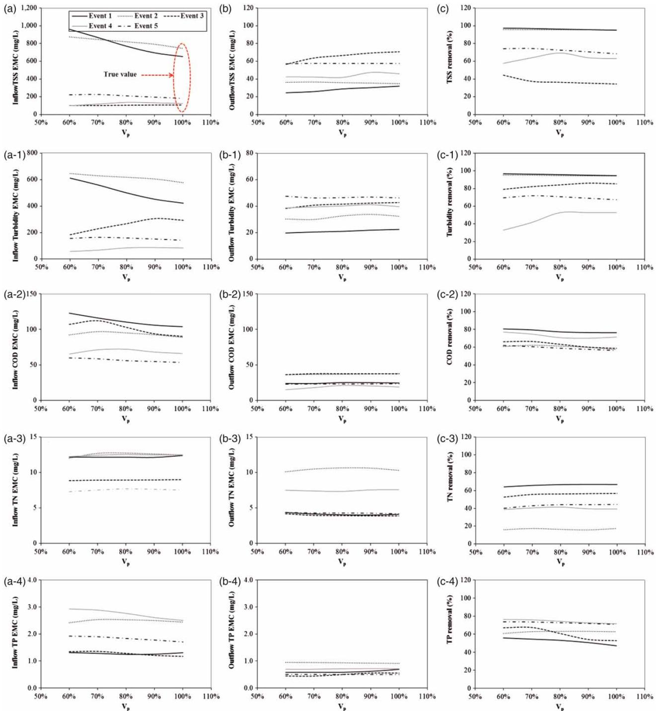
**Figure 3** | Change in EMCs and removal efficiency with respect to  $V_p$  (the return of base flow of the influent was implemented as the sampling end indicator; the data corresponding to 100% are true values).
