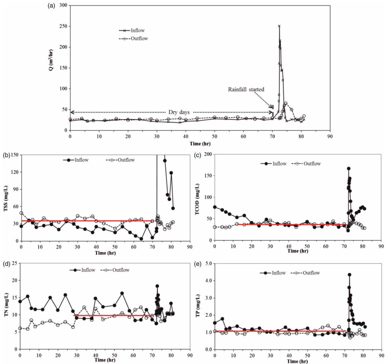
**Figure 5** | Hydrological condition and selected pollutants in the inflow and outflow during the period between storm events (the time when the inflow rate reached the base flow value was set as 0).
