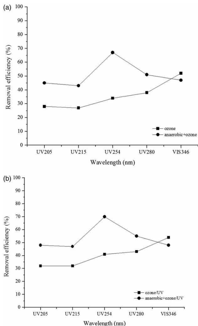
**Figure 3** (a) Removal efficiency in the different wavelengths on ozone and anaerobic + ozone (b) removal efficiency in the different wavelengths on ozone/UV and anaerobic + ozone/UV.
