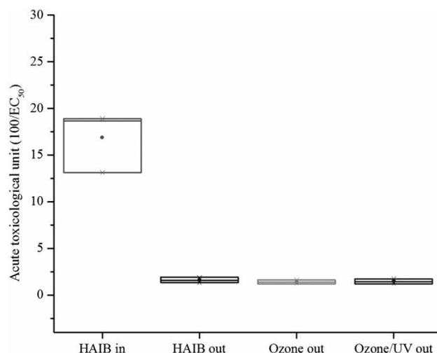
**Figure 4** | Acute toxicological units after ozone and ozone/UV application (box indicates: mean and maximum–minimum values. HAIB<sub>in</sub> (EC<sub>50</sub>): 5.47–7.42%).
