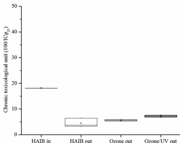
**Figure 5** | Chronic toxicological units after the treatments (box indicates: mean and maximum–minimum values). HAIB<sub>in</sub> (IC<sub>p25</sub>): 5.52%.
