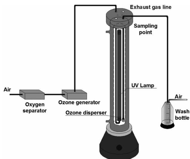
Figure 1 | Schematic diagram of the bench-scale oxidation reactor.
