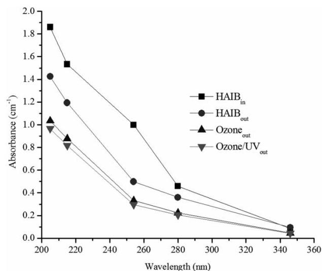
**Figure 2** | Values of absorbance in different wavelengths after treatments (dilution factor: 1:20).
