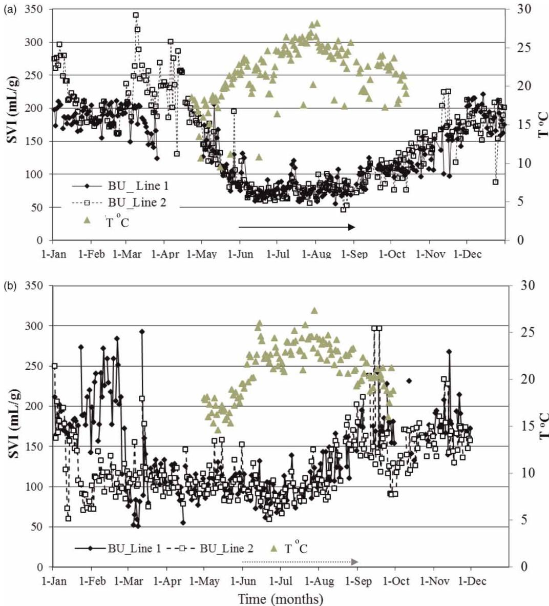
**Figure 1** | Sludge volume index data of the biological unit and inlet wastewater temperature in years (a) 2011 and (b) 2012 (solid arrow showing the cut-off period in 2011 and dotted arrow in 2012).
