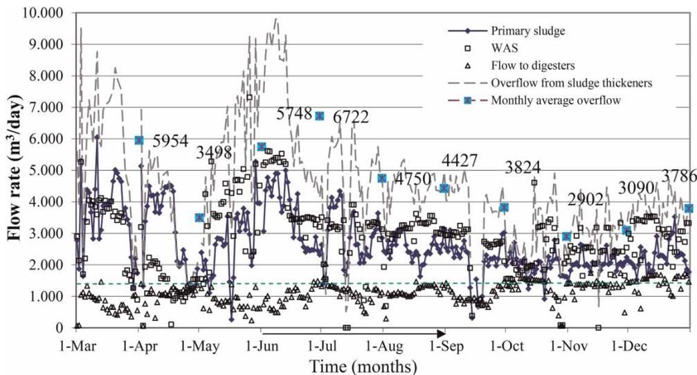
**Figure 3** | Flow rate data of the Konya WWTP on the sludge line between March and December 2011 (arrow showing the ARW's cut-off period and dotted line for sludge feeding design value).
