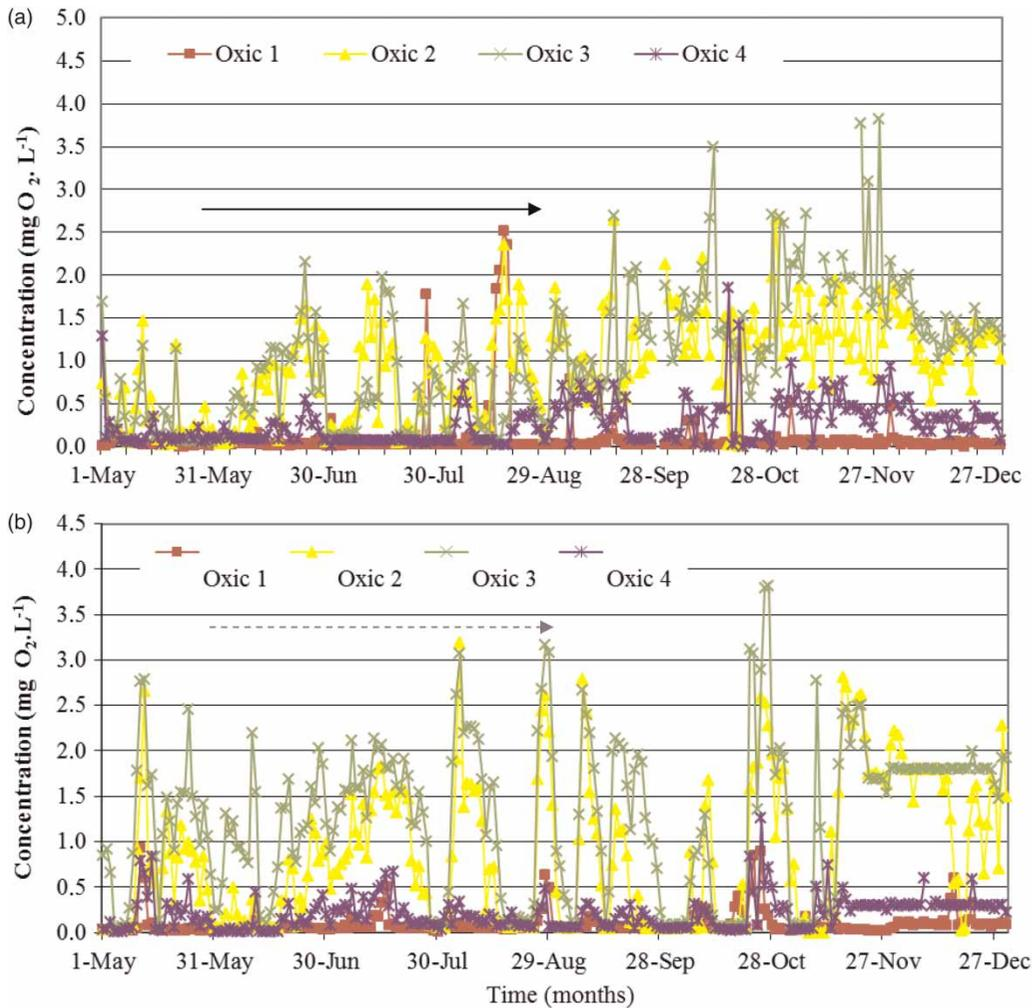
Figure 5 | BU Line-1 oxenic zones DO concentration profiles in 2011 (a) and 2012 (b) (solid line showing the cut-off period in 2011 and dotted arrow in 2012).
