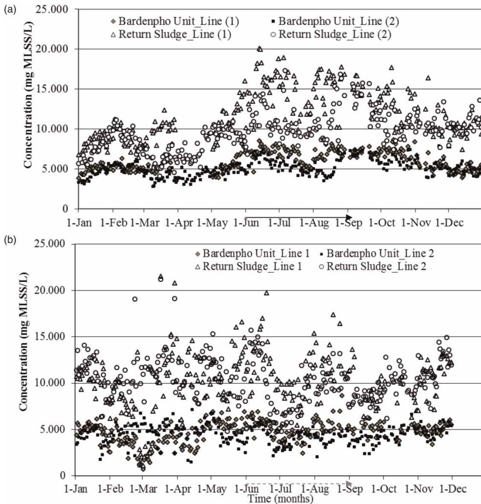
**Figure 2** | Suspended solids concentrations of BU and return sludge for the year of 2011 (a) and 2012 (b) (solid arrow showing the cut-off period in 2011 and dotted line in 2012).
