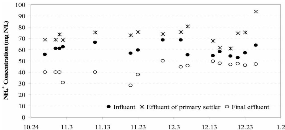
Figure 4 | Nitrogen concentration on the main flow line of WWTP during April–December 2011.
